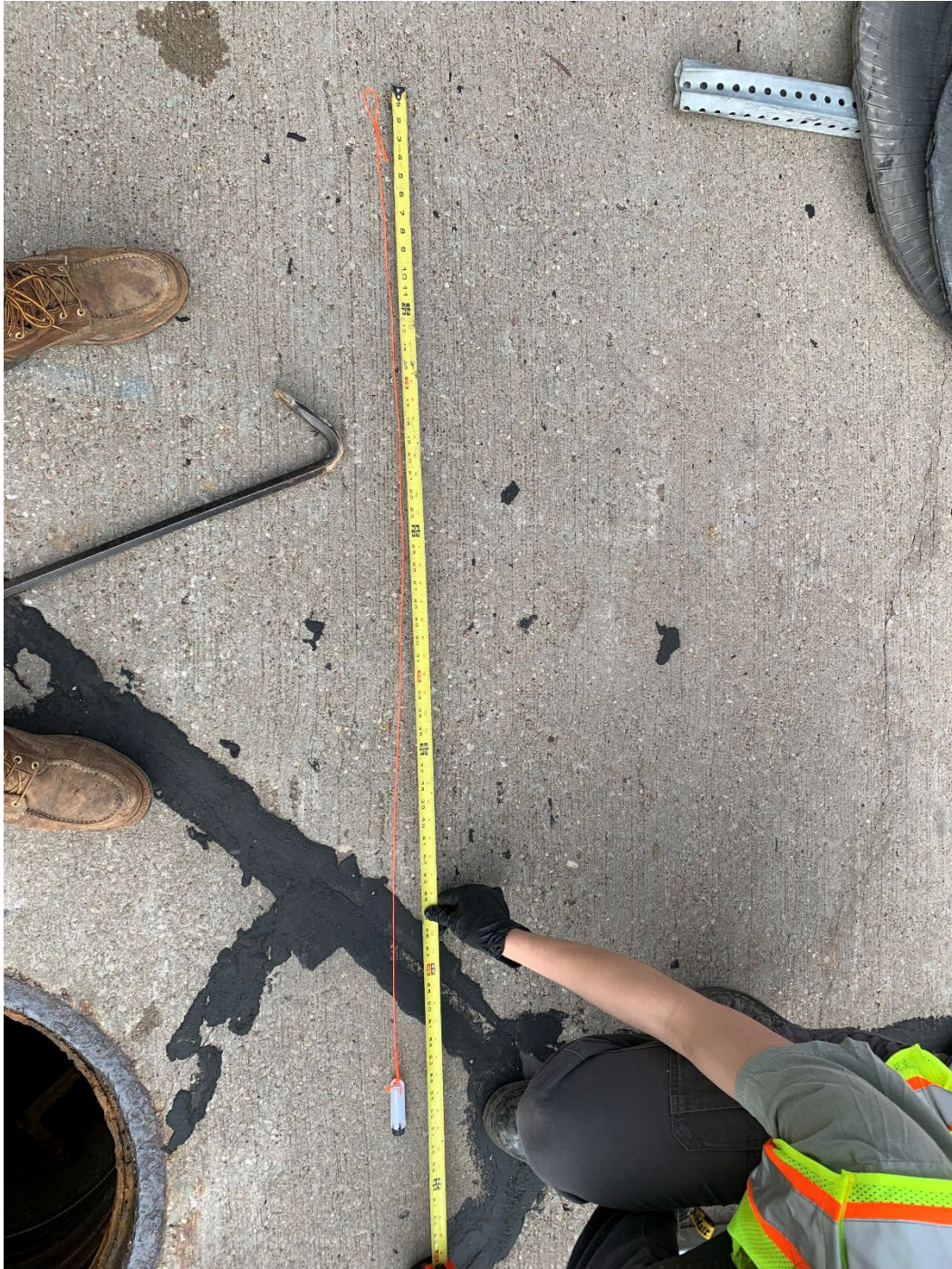
Photo 2: Measuring the string length to suspend the Beacon sampler at the appropriate depth.
