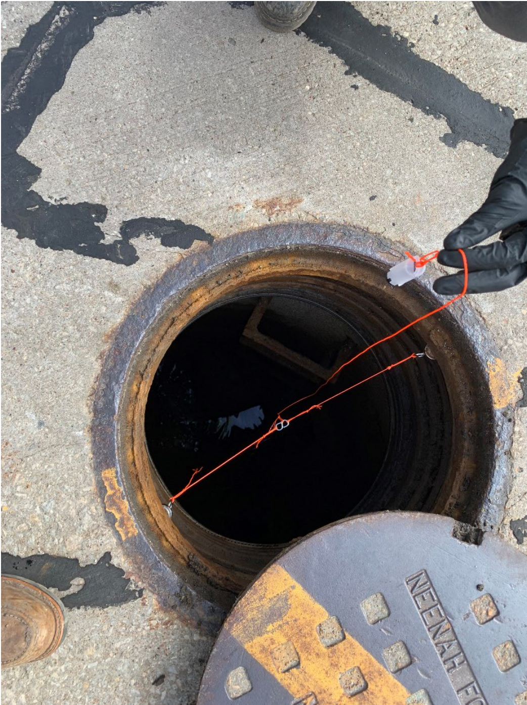
Photo 4: Beacon sampler ready for deployment with twisted mason line secured with neodymium magnets.
