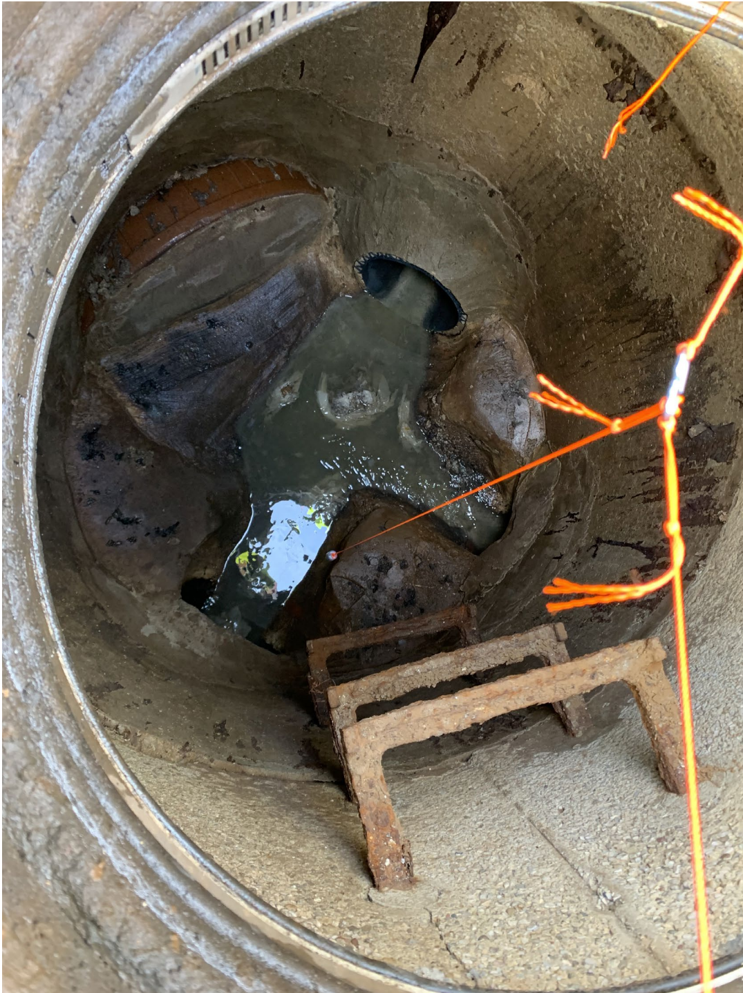
Photo 5: Beacon sampler suspended approximately one foot above the liquid level.
