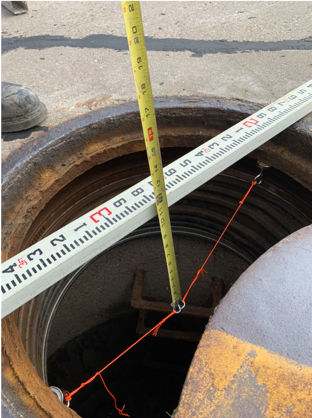
Photo 3: Measuring the magnet suspension connection depth to place the Beacon sampler at the appropriate depth.
