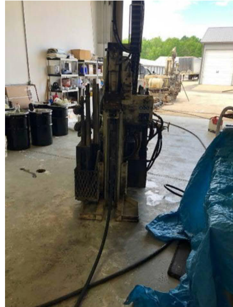
Photo #2 Photograph of injection boring installation and subsequent amendment injection.
