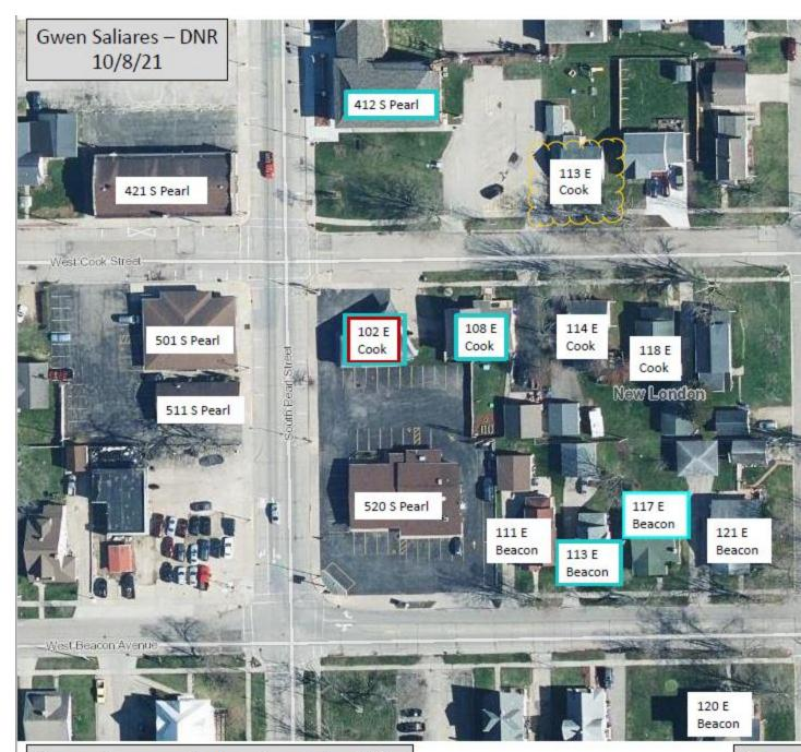
Properties screen-in based on being 100 ft from CVOC impacted soil and/or 100 ft from monitoring point with CVOCs above Enforcement Standards
