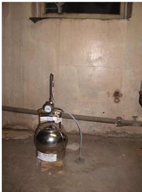
Photograph No.: 22 Photographer: Naren Babu Orientation: North TDD Number: TO-05-11-03-0007 Contract: EP-S5-10-10, OTIE Date: April 20, 2011 Site Name & Location: Sandies Dry Cleaning Site, Little Chute, Outagamie County, Wisconsin. Subject: View of the sub-slab soil-gas, SDC-SG-02, sample collected from Sandies
