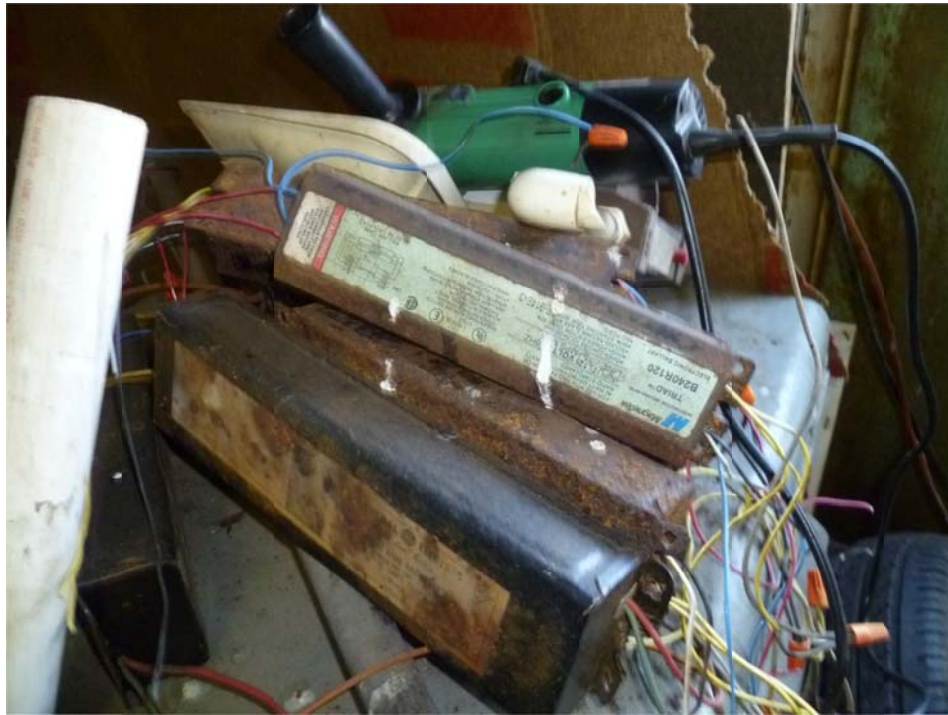
Photograph No.: 7 Photographer: Naren Babu Orientation: Looking Down TDD Number: TO-05-11-03-0007 Contract: EP-S5-10-10, OTIE Date: April 7, 2011 Site Name & Location: Sandies Dry Cleaning Site, Little Chute, Outagamie County, Wisconsin. Subject: Electrical ballasts found inside Sandies Dry Cleaners which may contain PCBs
