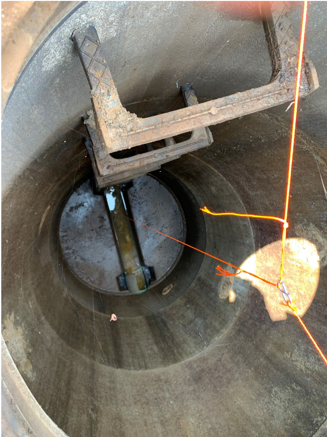
Photo 4: Beacon sampler deployed with twisted mason line secured with neodymium magnets.
