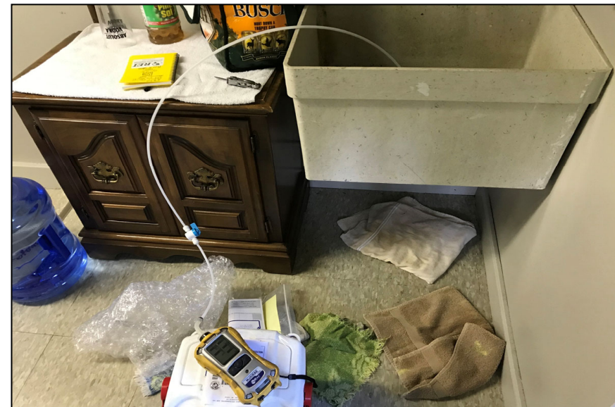
Purging line and collecting field measurements
