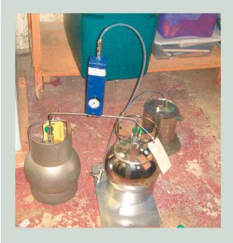
A sub-slab vapor sampling system is usually in place for a day or two during the sampling process. The metal canisters (foreground) collect the vapor sample from the port (smaller canister in back of photo). The same canisters can be used to collect indoor air samples.
