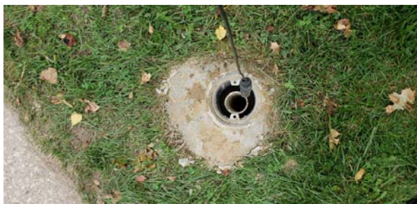
Placement of Pressure Transducer/Data Logger for Slug Test
