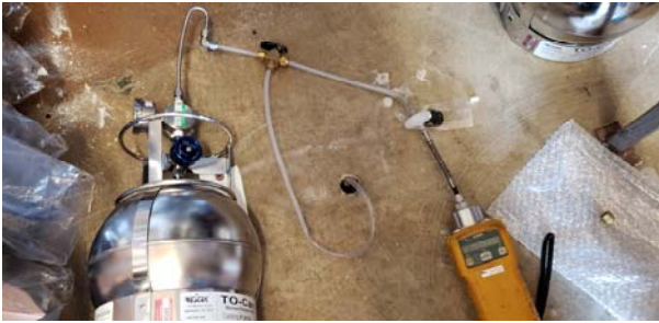
Connecting Vapor Sampling Train
