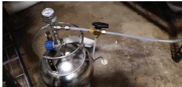
Purge and Sampling for Sub-Slab Vapor
