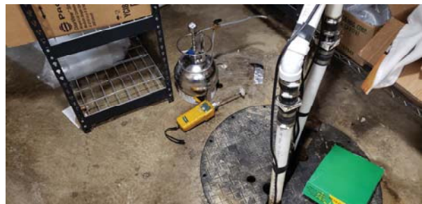
Sampling in the Basement of the Restaurant Building Next to a Sump Manhole
