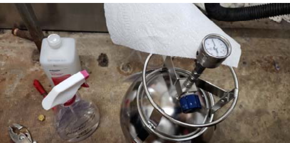
Spray Isopropyl Alcohol on the Paper Towers over the Sampling Train for Potential Leakage Check (QC)
