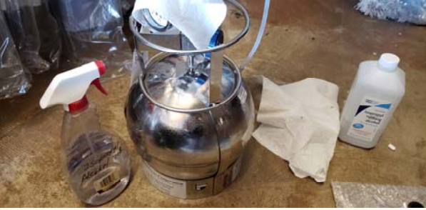
Sub-Slab Vapor Sampling Train Assembled & Ready for Spraying of Isopropyl Alcohol
