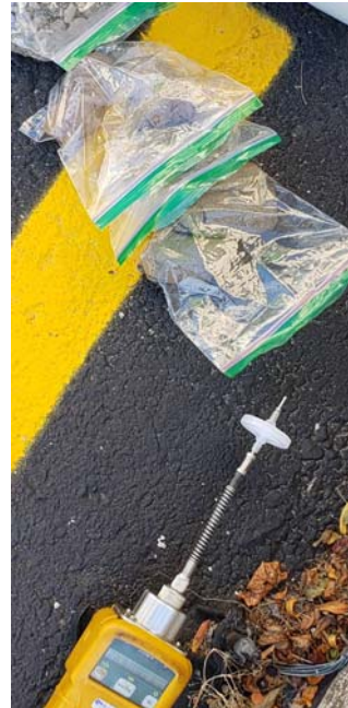
Soil Core Head-Space VOC Testing with PID
