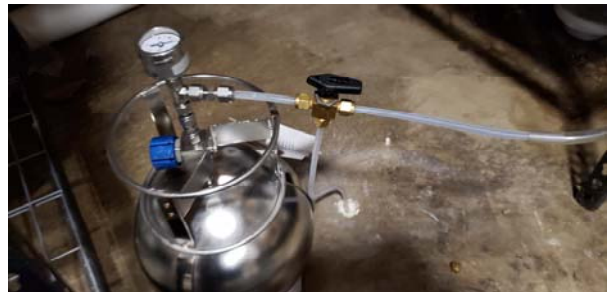
Purge and Sampling for Sub-Slab Vapor
