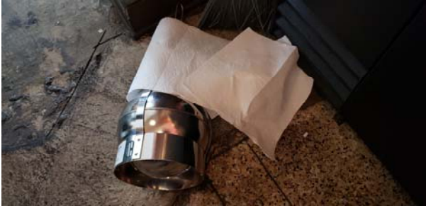
Sub-Slab Vapor Sampling Train Covered with Paper Towels Sprayed with Isopropyl Alcohol
