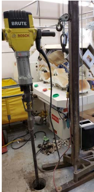
Indoor Soil Boring with Probing
