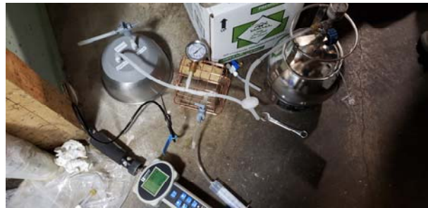
Shut-In Test for the Sampling Train
