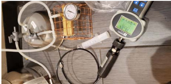
Supply Helium to the Shroud Covered on the Sampling Port
