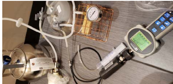
Test the Sampling Train for Helium Leakage
