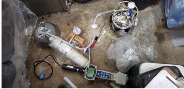
Configuration for Sub-Slab Vapor Sampling
