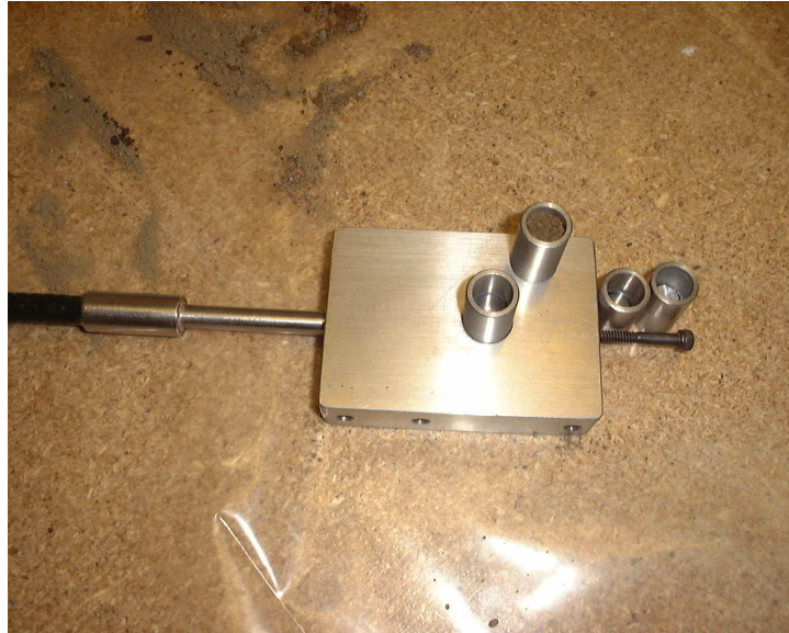
Figure 4. Sapphire-windowed sample cups with fiber optic attached. Parabolic mirror inside emulator turns beam into cup.
