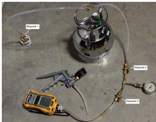
Figure 1. Example of Sub-Slab Sampling and Leak-Test Setup
