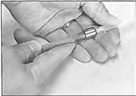
Figure 1. Attaching tubing to the sampling implant.
