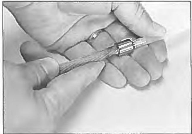
Attaching polyethylene tubing to the sampling implant.
