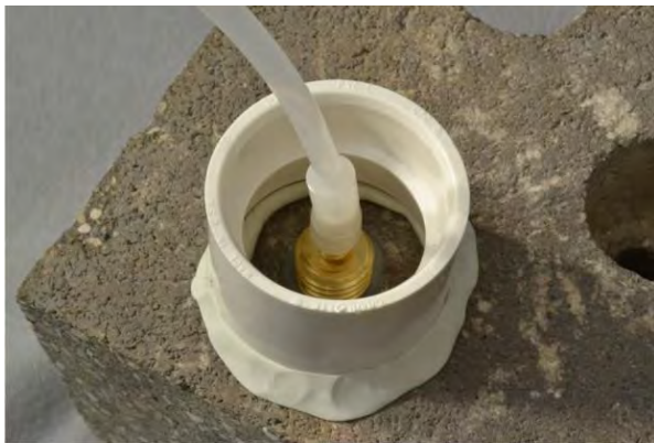
Figure 6. Water dam used for leak detection
