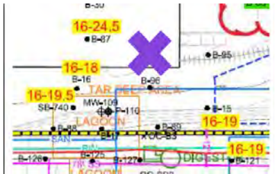
From Figure 7: Observed Tar (16-20' BGS), 06/04/20
