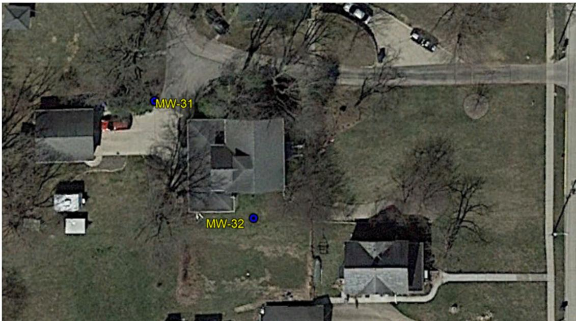
Soil samples were collected from the surface to 40 feet in the soil boring drilled for installation of monitoring well MW-31 and from the surface to 35 feet in the soil boring drilled for installation of monitoring well MW-32. Soil samples were collected for field screening with a
