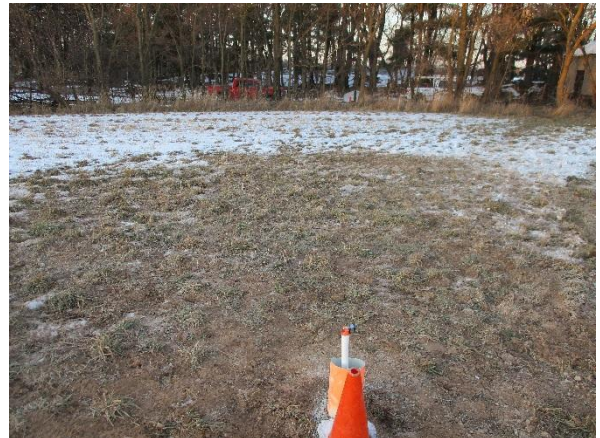
Photo #4 Photo looking south at MW-9 depicting 1-inch well inside 6-inch outer casing. MW-6 is located 100 feet to north.
