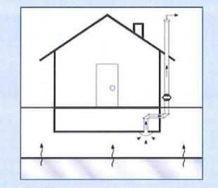
If potentially harmful chemical vapor intrusion is detected in a home or business, the most common solution is to install a sub-slab depressurization system. This system captures and redirects soil vapors from below the building foundation before they enter the indoor air. Vapors are vented outside of the building where they disperse into the air and are rendered harmless.
