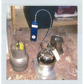
A sub-slab vapor sampling system is usually in place for a day or two during the sampling process. The metal canisters (foreground) collect the vapor sample from the port (smaller canister in back of photo). The same canisters can be used to collect indoor air samples.
