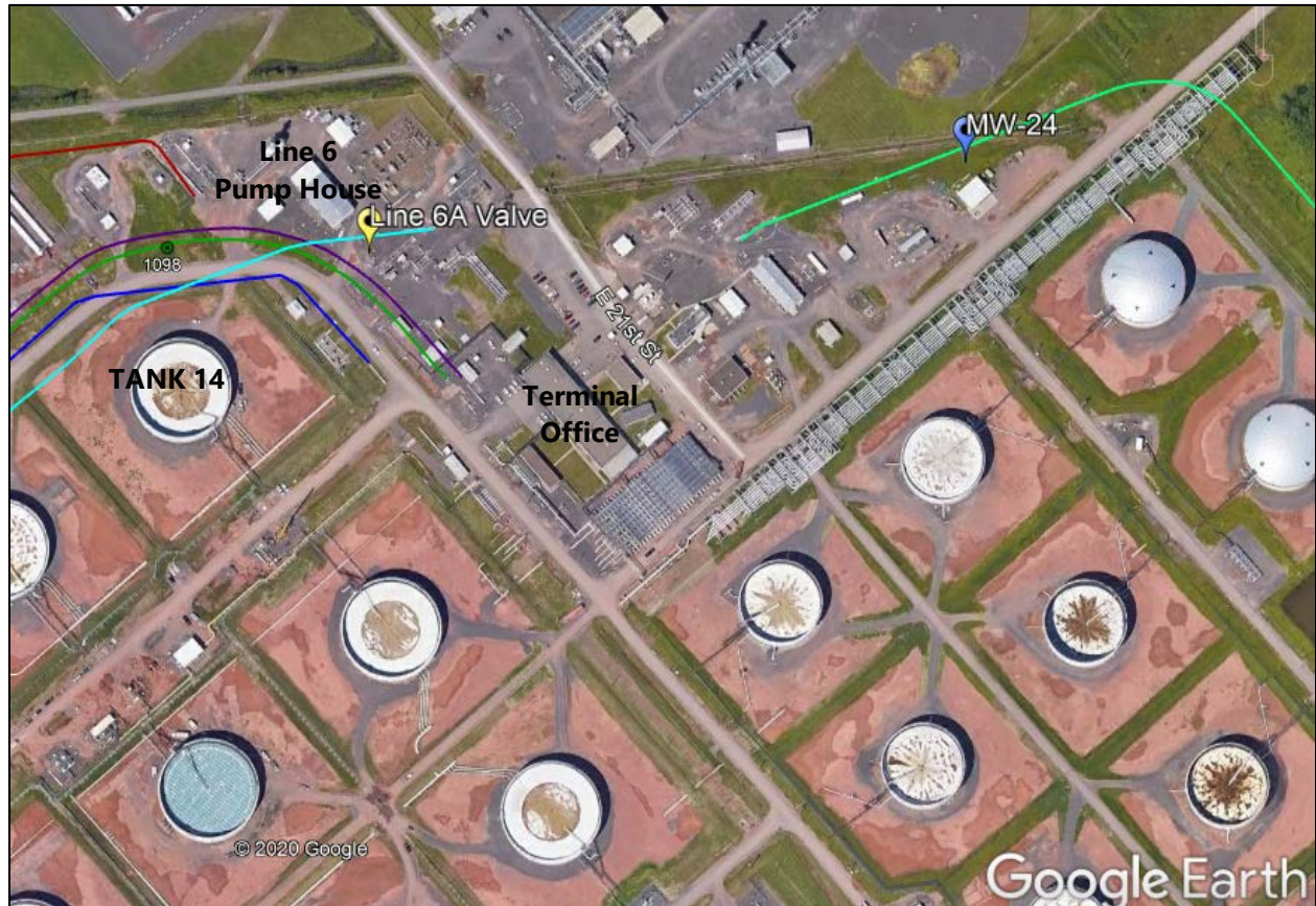
Figure 1, Site Location: The north-central side of the Enbridge Superior Terminal, the Line 6A Valve excavation (yellow pin; top left corner), and Terminal monitoring well MW-24 (blue pin; top right corner). Image from Google Earth.
