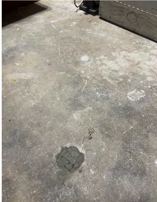
Photo 7: Sub-slab sample point SSV-03 in the 1233 12th Avenue building following installation of the temporary cement cap. Previous SS-3 sample location visible. 3/22/2023.
