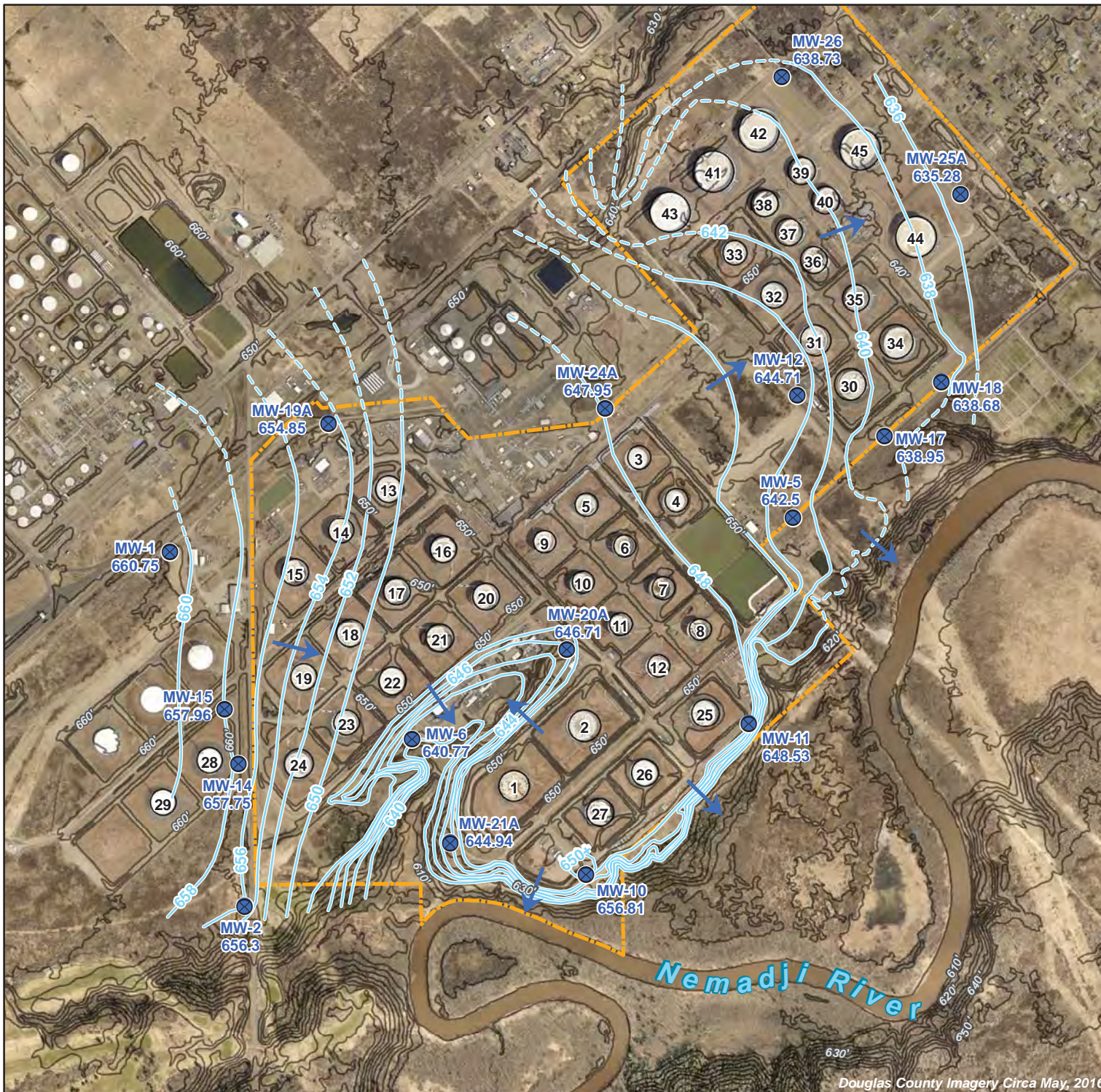
Feet 1 Inch = 1,000 Feet Figure 3 SPRING 2017 SHALLOW GROUNDWATER ELEVATION CONTOURS Superior Terminal Enbridge Energy, L.P. Superior, Wisconsin
