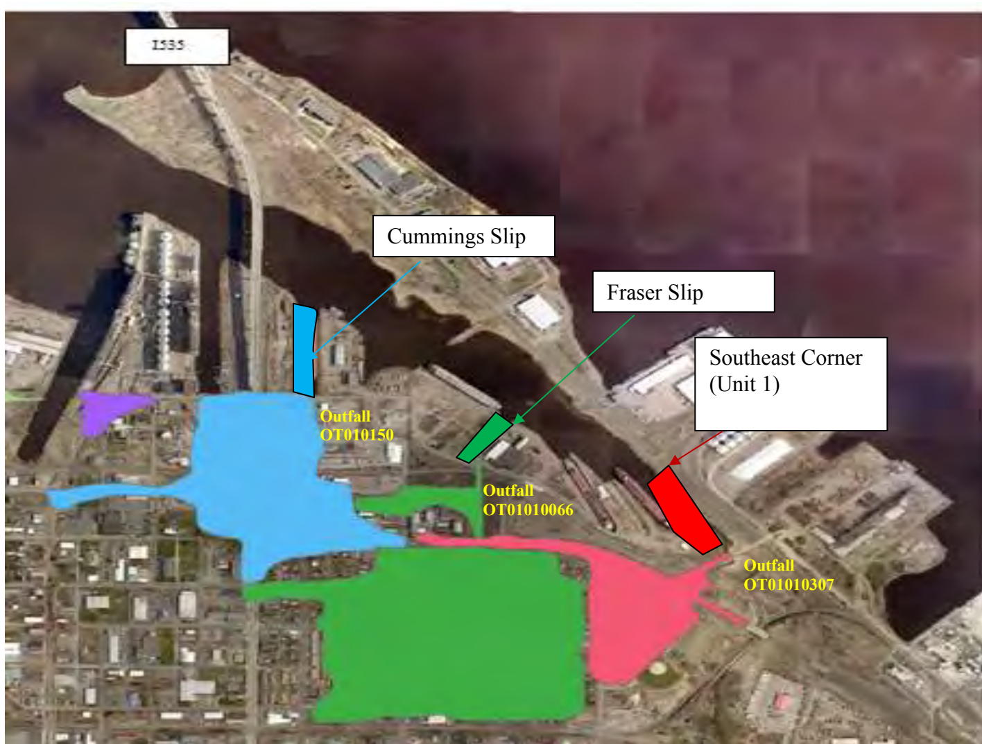
Fig. 7 Drainage area of the MS4 and location of major outfalls in Howards Bay (City of Superior, 2014)
