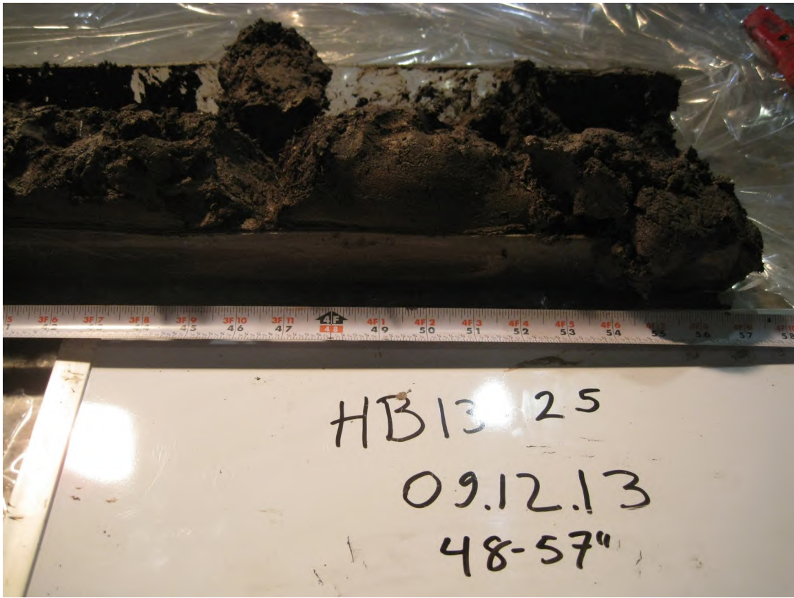
Core HB13-25: 48 to 57 inch depth interval. Brown clay. See core log for full description. Photo by ARCADIS 09/12/2013
