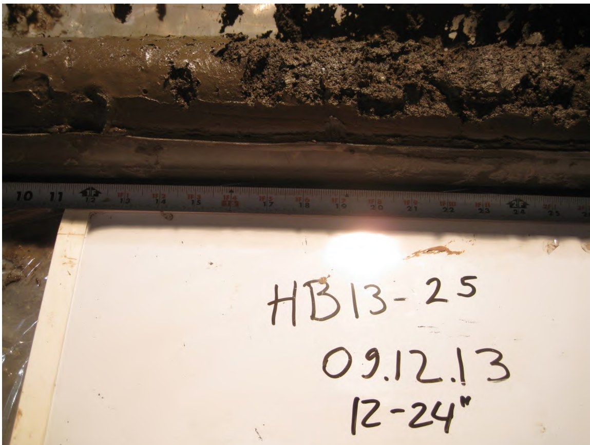
Core HB13-25: 12 to 24 inch depth interval. Grey brown silt. See core log for full description. Photo by ARCADIS 09/12/2013.
