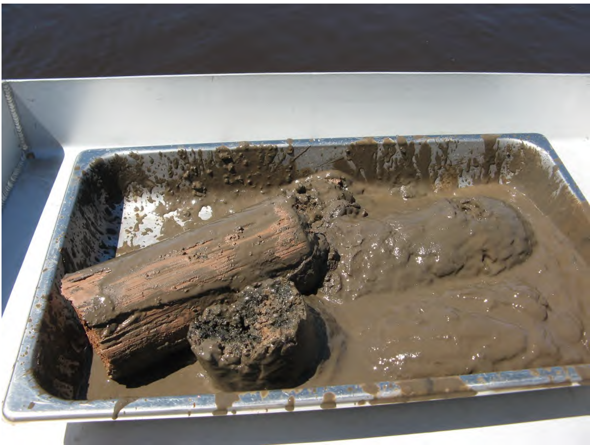
Extraction of core HB17-17 into pan. (Photo 1 of 3): Top to right. Note plug of dense red clay from core bottom (left)
