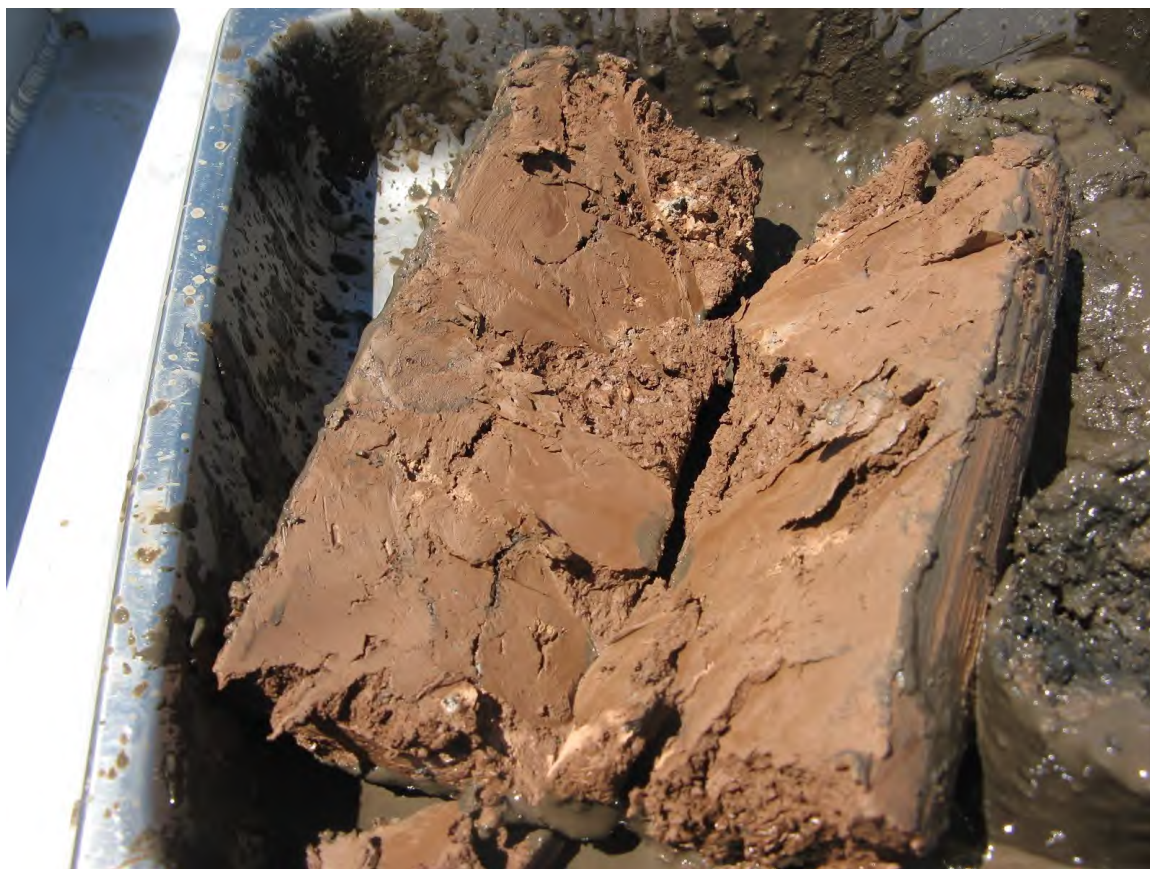
Extraction of core HB17-17 into pan. (Photo 3 of 3): Close-up of red clay plug split lengthwise.
