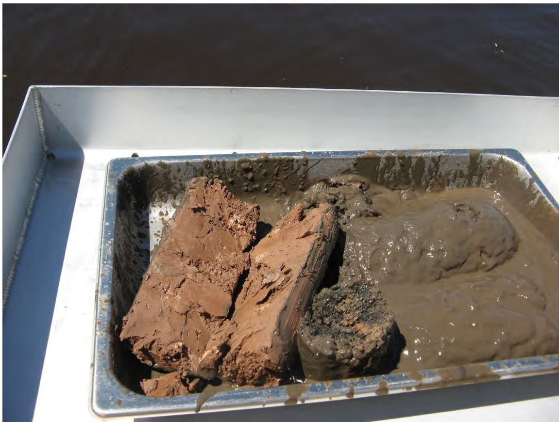
Extraction of core HB17-17 into pan. (Photo 2 of 3): Red clay plug split lengthwise.
