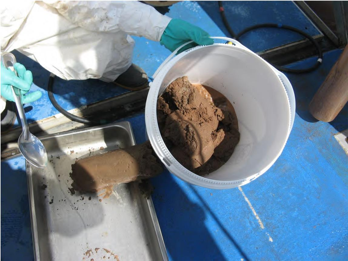
Contents of Core 1 of 5 at HB17-07 for USACE treatability sample; bucket contains sand from top of core , pan at right has 12 inches of brown silty clay from bottom of the core tube. Photographed by J. Graham 06/20/2017 with Cannon Power Shot A710.
