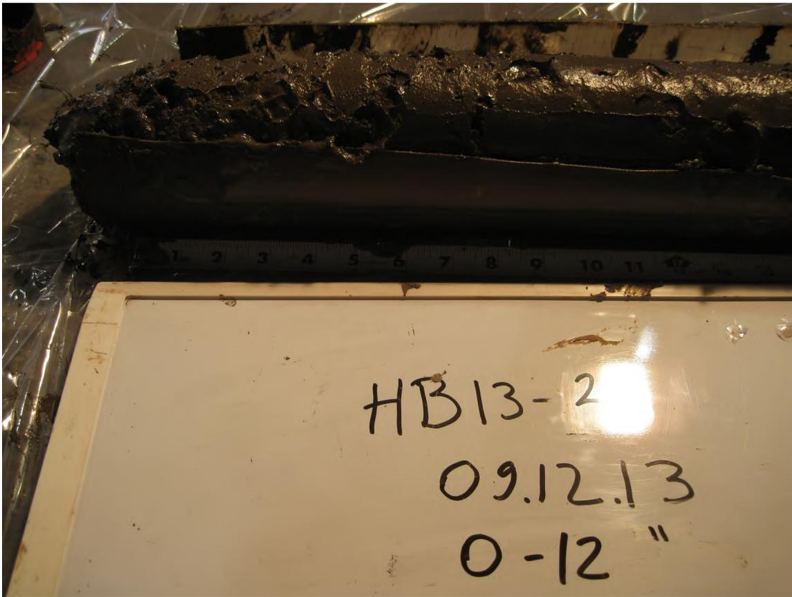
Core HB13-25: 0 to 12 inch depth interval. Grey Brown Silt. See core log for full description. Photo by ARCADIS 09/12/2013
