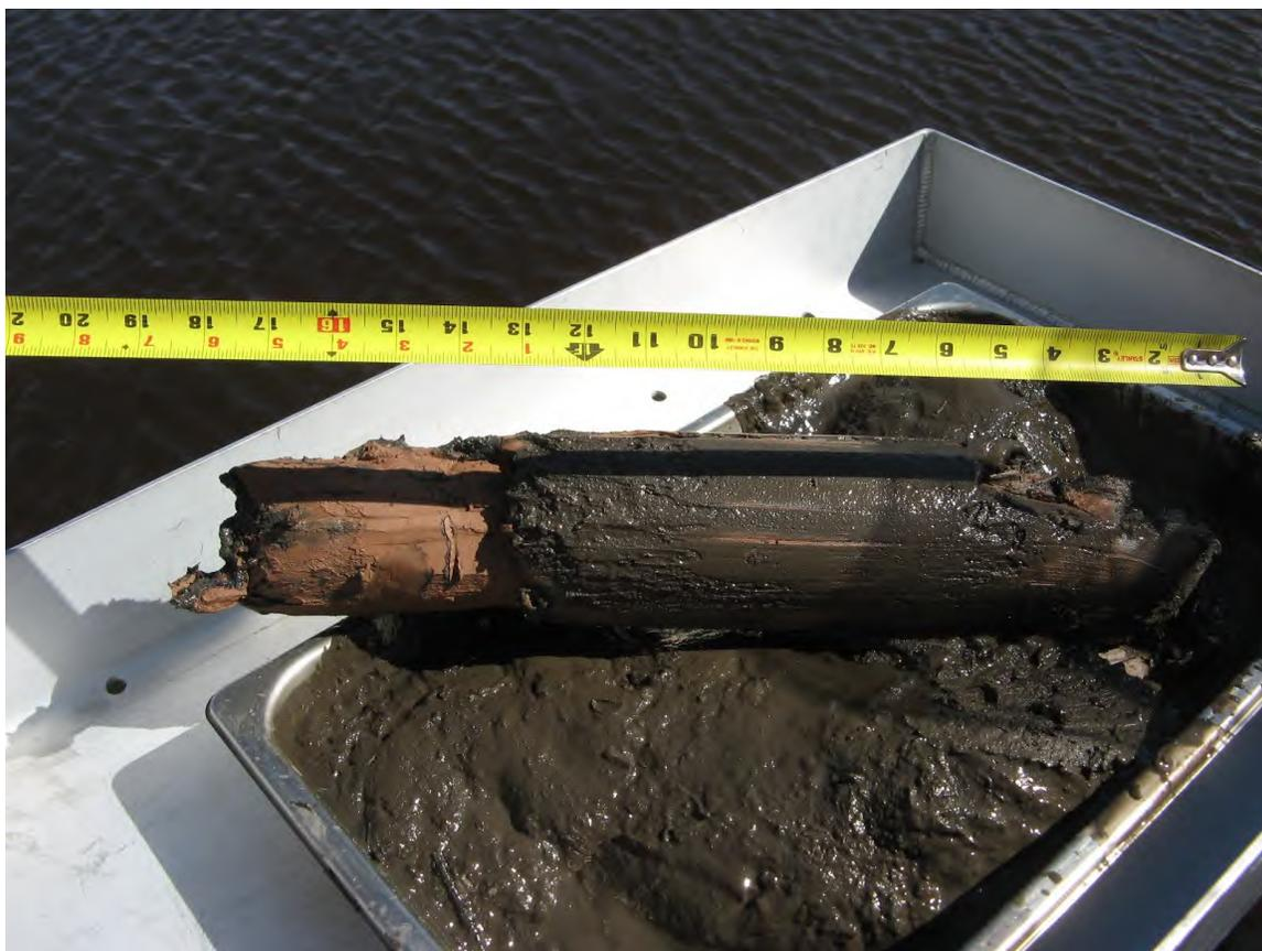
Extraction of core HB17-21, note red clay plug from bottom of core.
