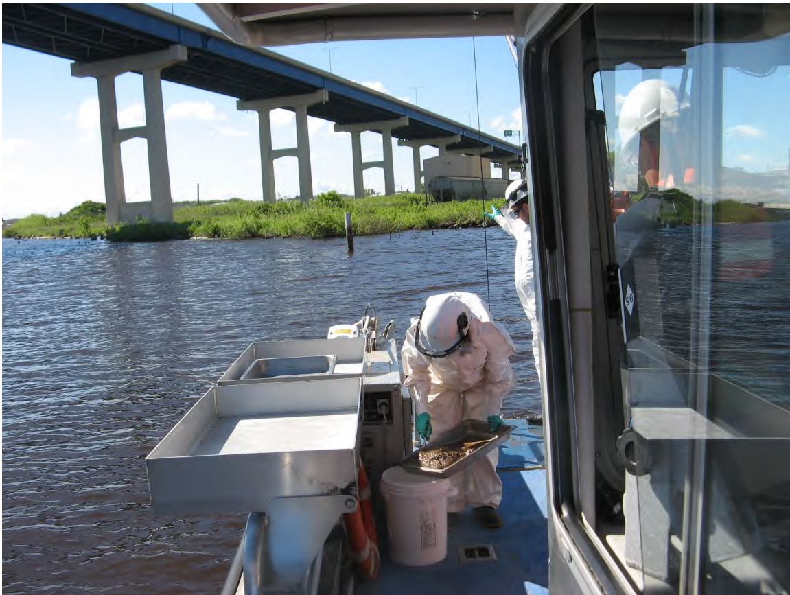
Ponar grab sample for treatability testing at HB17-01
