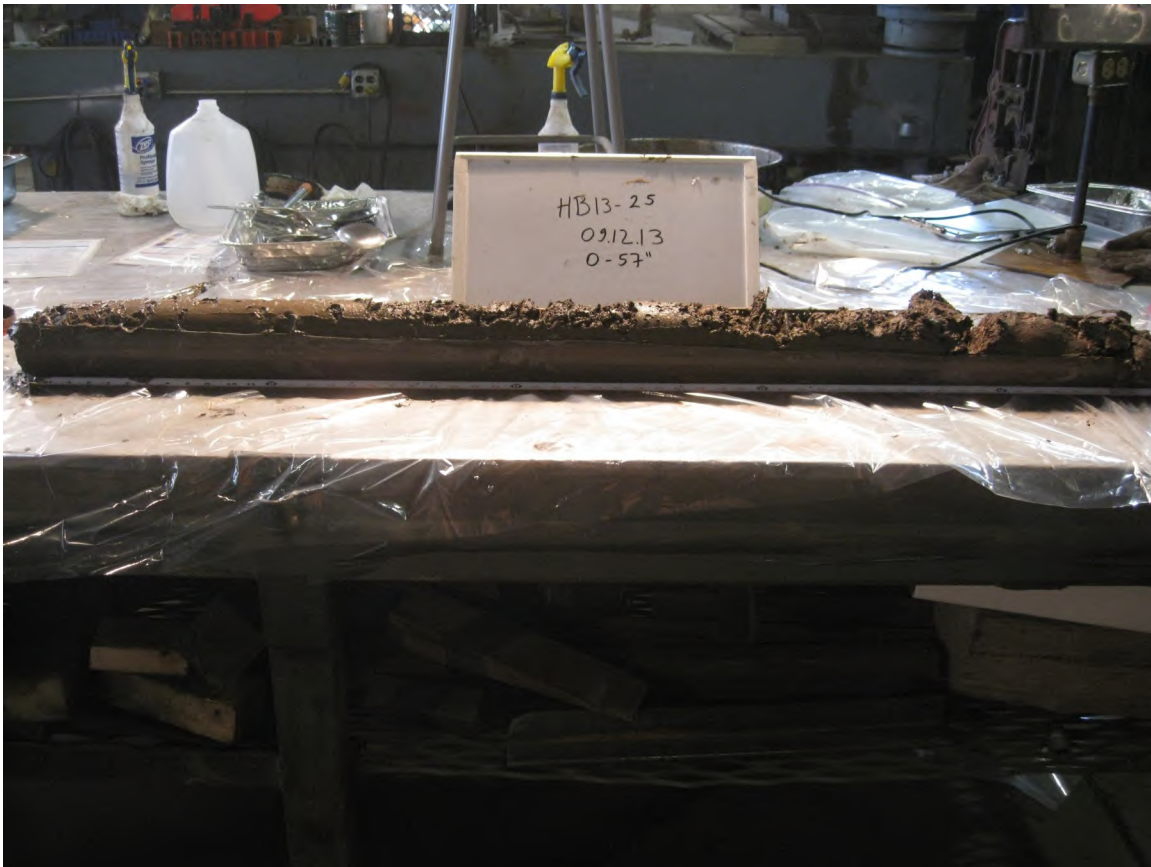
Full profile—no flash. Top is to left. Top is grey brown silt. See core log for full description. Photo by ARCADIS 09/12/2013.
