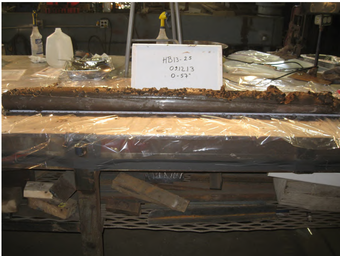
Full profile—with flash. Top is to left. Top is grey brown silt. See core log for full description. Photo by ARCADIS 09/12/2013.
