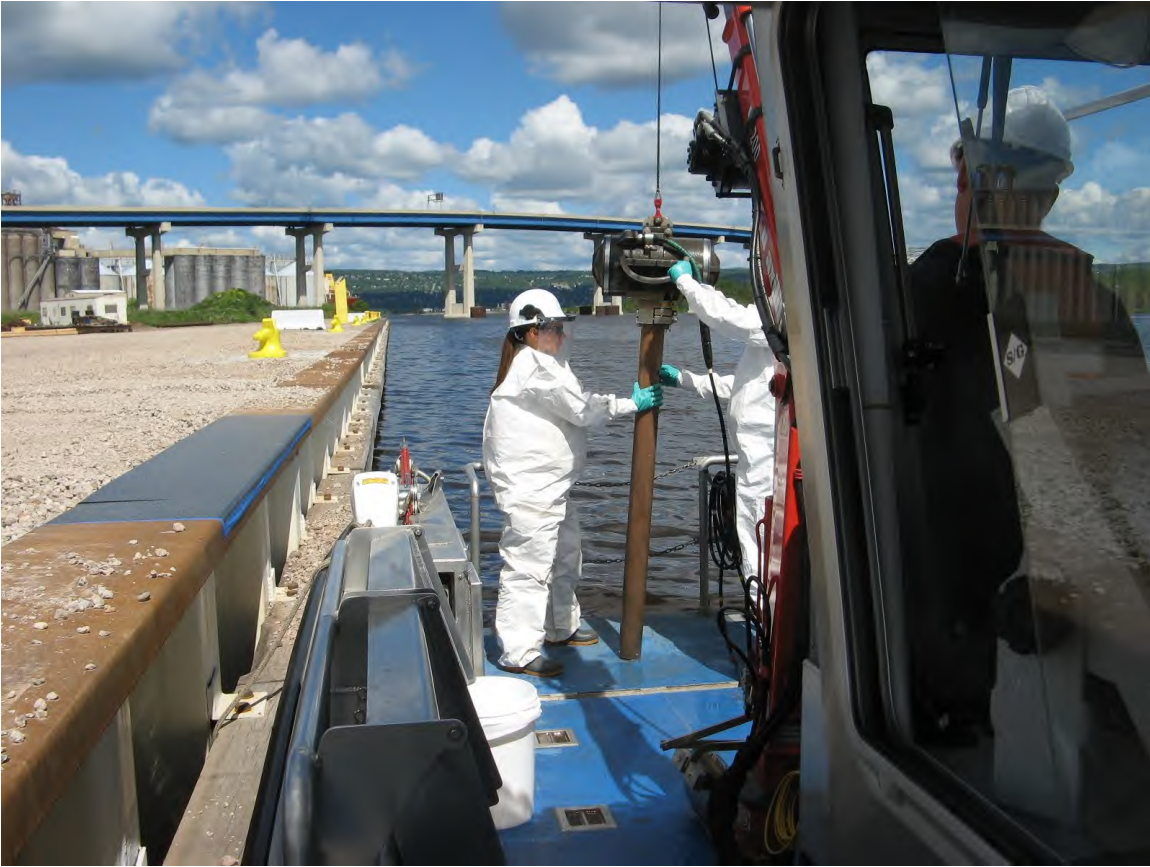
Typical Core at HB17-07: Cores at this location were collected off right side of the boat using boom arm of crane. Photographed by J. Graham 06/20/2017 with Cannon Power Shot A710.
