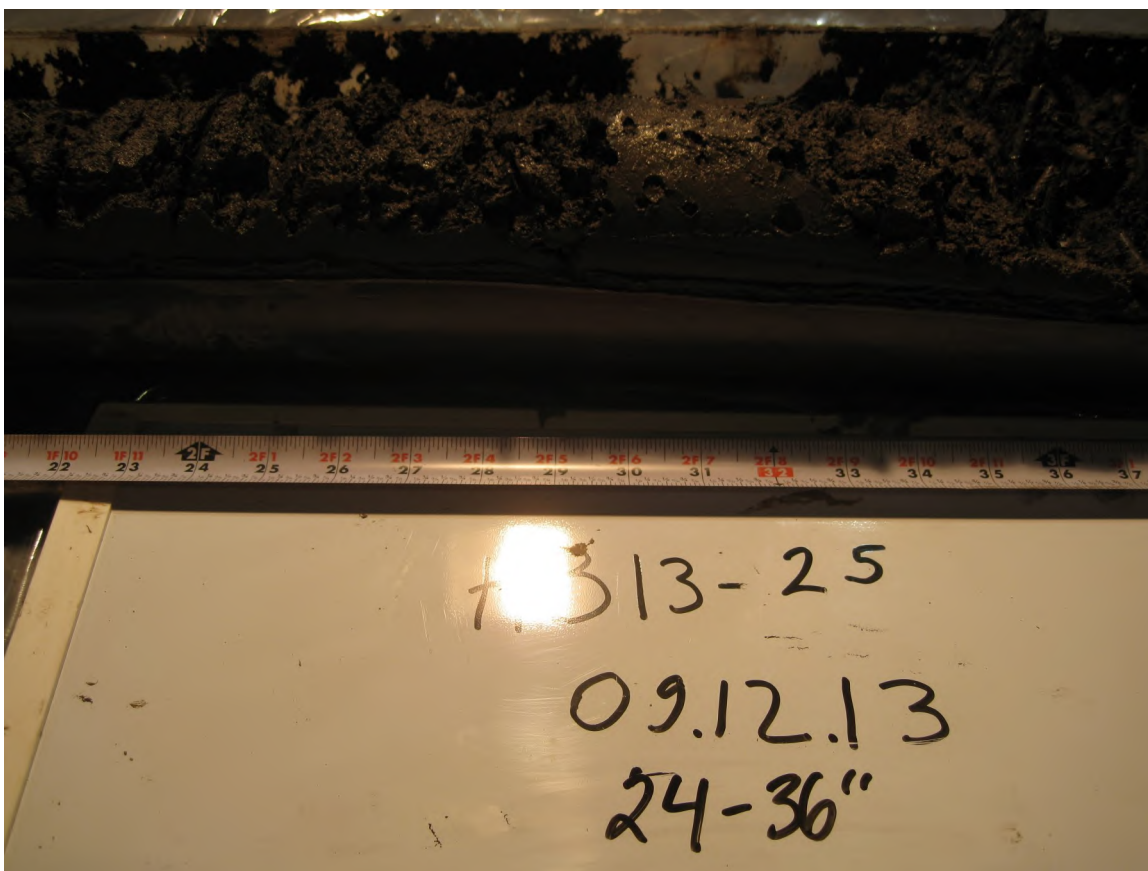
Core HB13-25: 24 to 36 inch depth interval. Grey Brown Silt. See core log for full description. Photo by ARCADIS 09/12/2013
