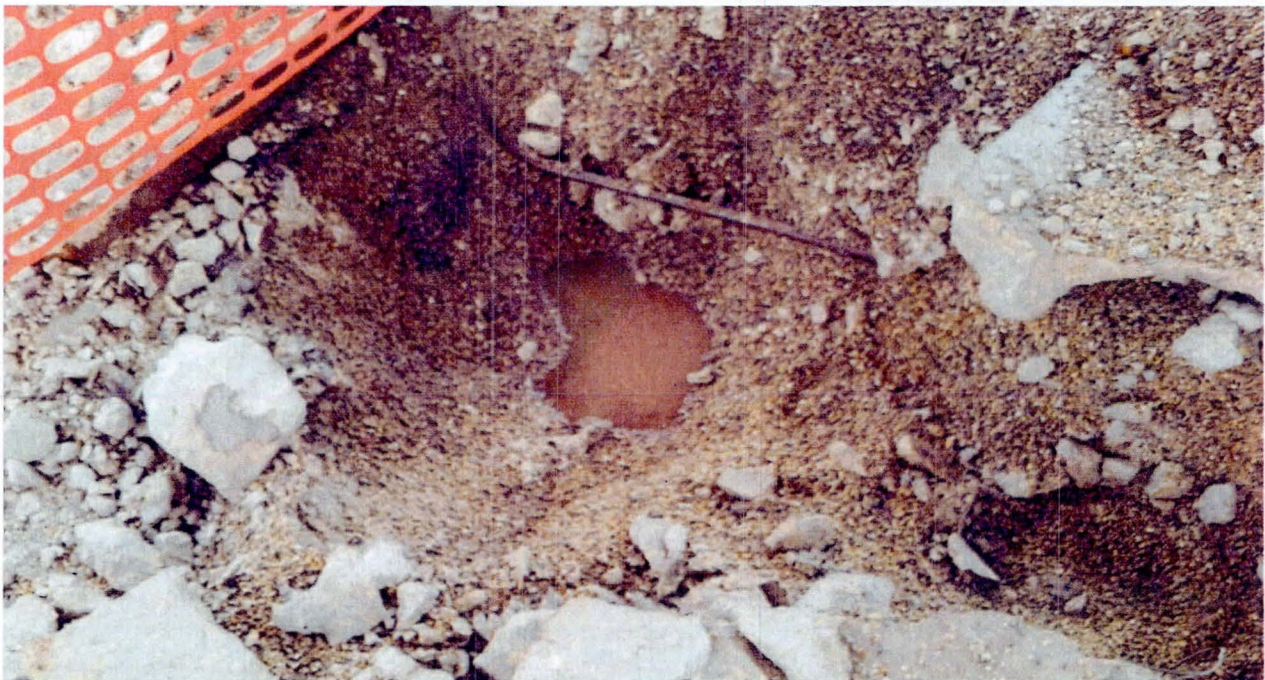
PHOTO 11 – PHOTOGRAPH OF SOIL SAMPLE COLLECTED BENEATH DISPENSER 4, SHEEN ON WATER.
