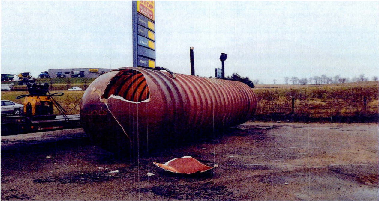
PHOTO 3 – PHOTOGRAPH OF ONE (1) 12,000-GALLON FIBERGLASS UNDERGROUND STORAGE TANK
