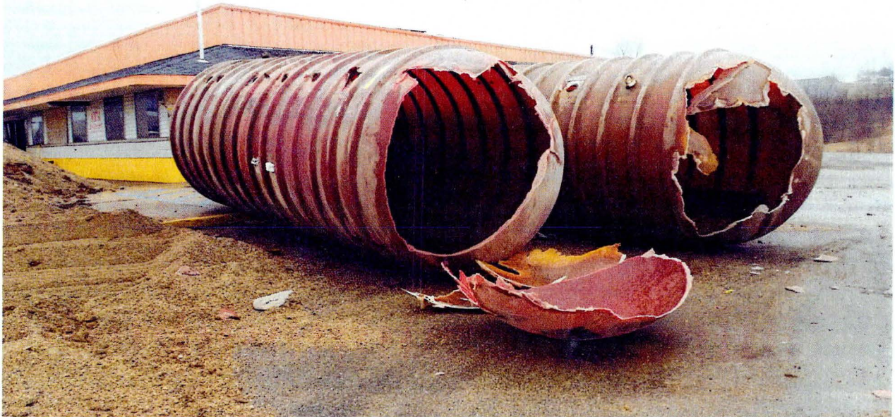
PHOTO 1 - PHOTOGRAPH OF ONE (1) 8,000-GALLON AND ONE (1) 12,000-GALLON FIBERGLASS UNDERGROUND STORAGE TANK
