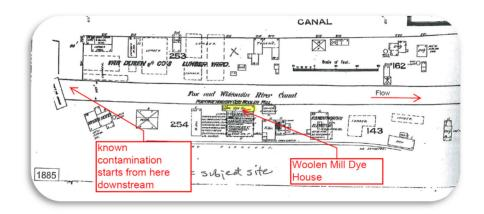
Accounts from local residents on the canal Ad Hoc committee indicate that the canal water became blue or red, depending on the color the mill was dying socks on a given day. Textile dyes can contain cadmium, chromium, copper, lead, mercury, and zinc based on publication EPA-600/2-78-098 *Textile Dyeing Wastewaters* (EPA, 1978).
