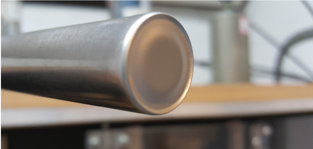
Condition: poor; heavy pitting, replace horn.
