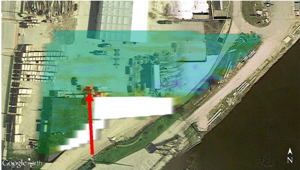
Figure 1- InPhase 5k (Metallic Features 2-3 Meters in Depth)
