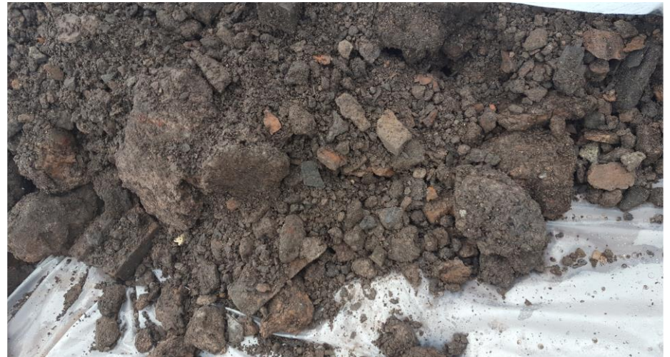
Petroleum impacted material from excavation in stockpile.
