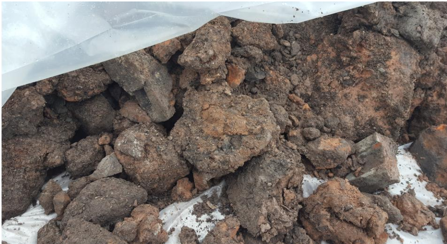
Petroleum impacted material from excavation in stockpile.
