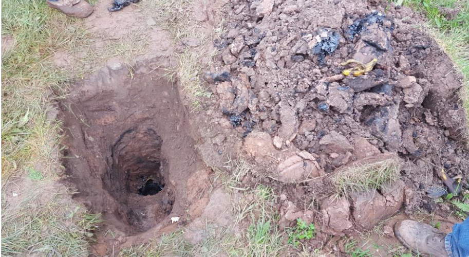
Boring with unknown petroleum product on south side of site.
