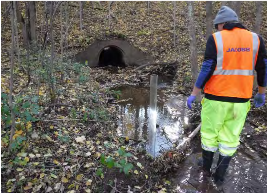
Manual coring at ML-SD-38 photo 1.JPG
