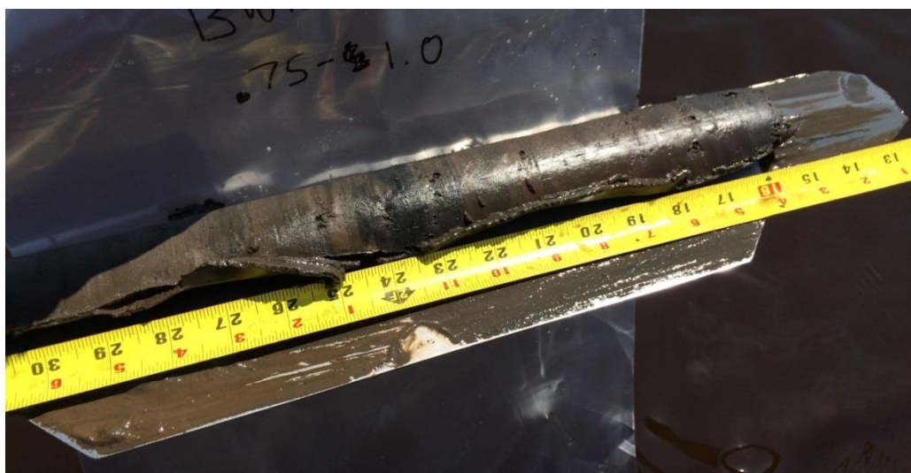
Photo showing discrete sample collected with Russian Peat Borer.
