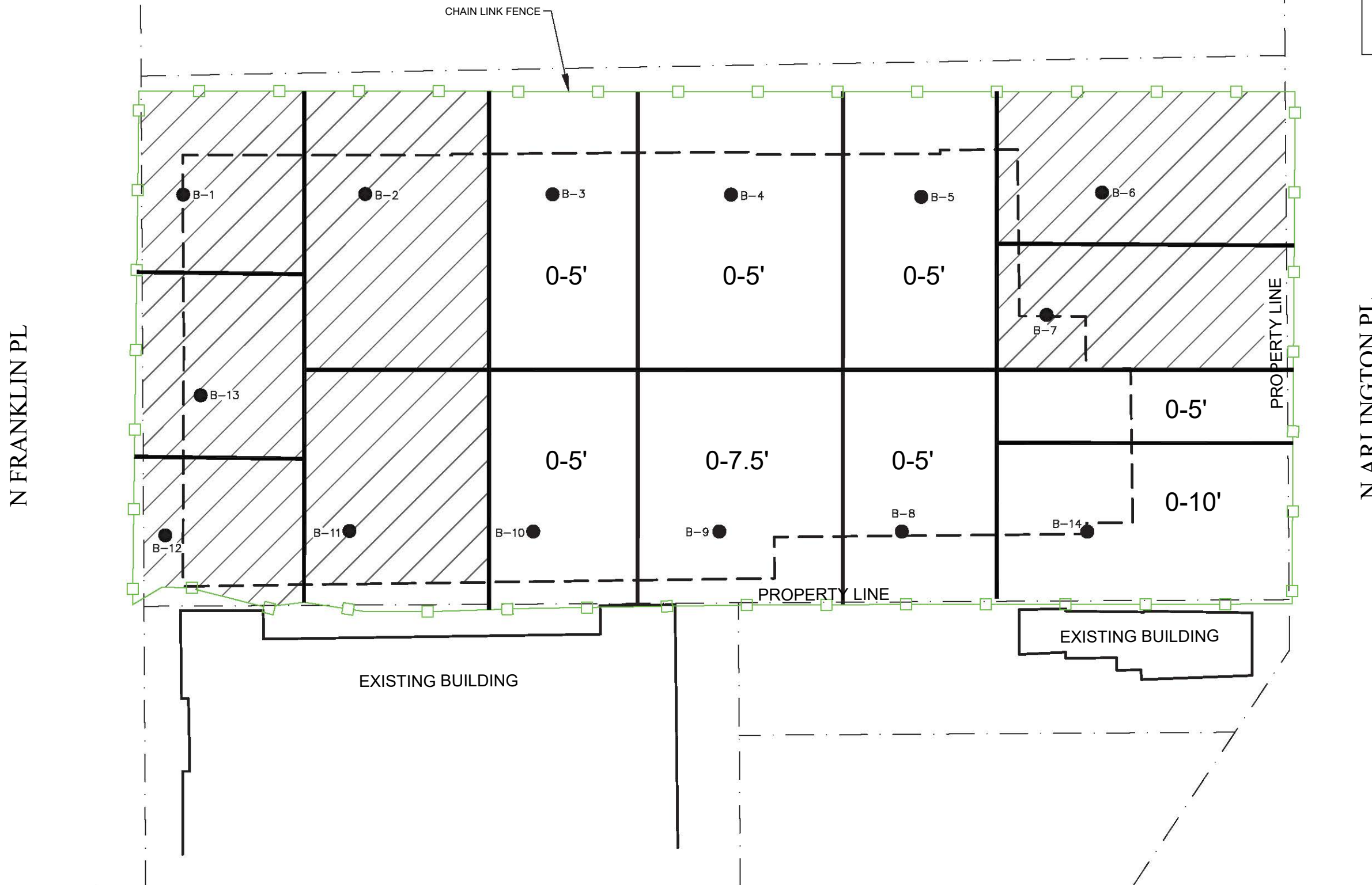
FIGURE 4 LOCATION OF SOIL RCL EXCEEDANCES BOYS & GIRLS CLUB 1632 N FRANKLIN PLACE MILWAUKEE, WISCONSIN
