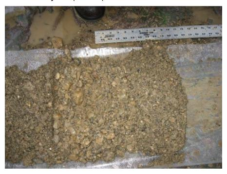
10 -15 feet SAND, medium to very coarse, little granules to medium pebbles, subround to subangular, trace silt; poorly sorted, wet, grayish brown (10YR5/2).
