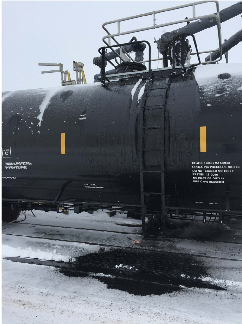
Photo 2: Looking east and standing on the west side of Track 3. The released product rolled down the side of the railcar and mostly dripped into containment.
