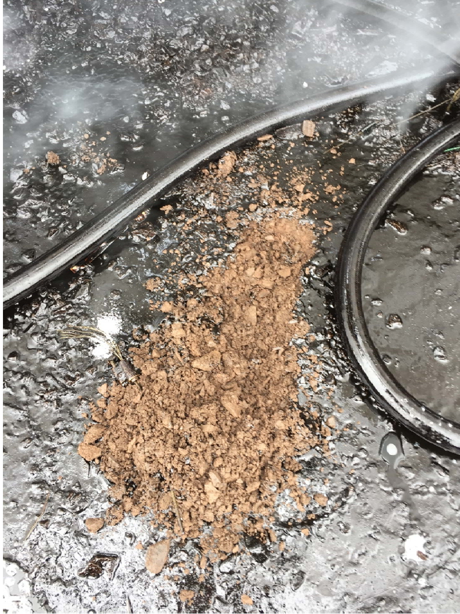
Photo 6: A gentle toe drag was done through the product to gauge its thickness.
