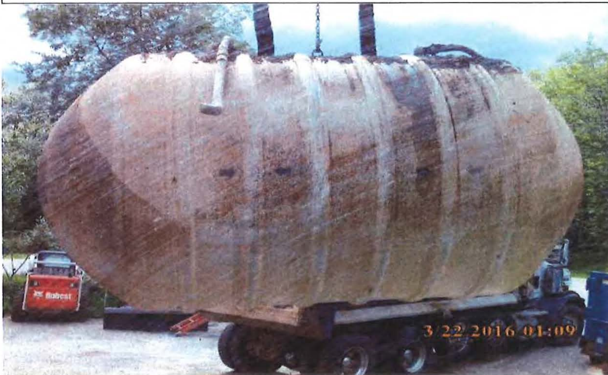
PHOTO 2 - PHOTOGRAPH OF THE 4,000-GALLON UST
