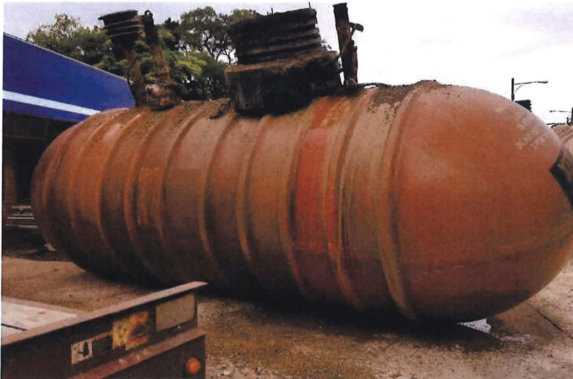
PHOTOGRAPH OF THE 2 ND 8,000-GALLON UNLEADED GASOLINE UST
