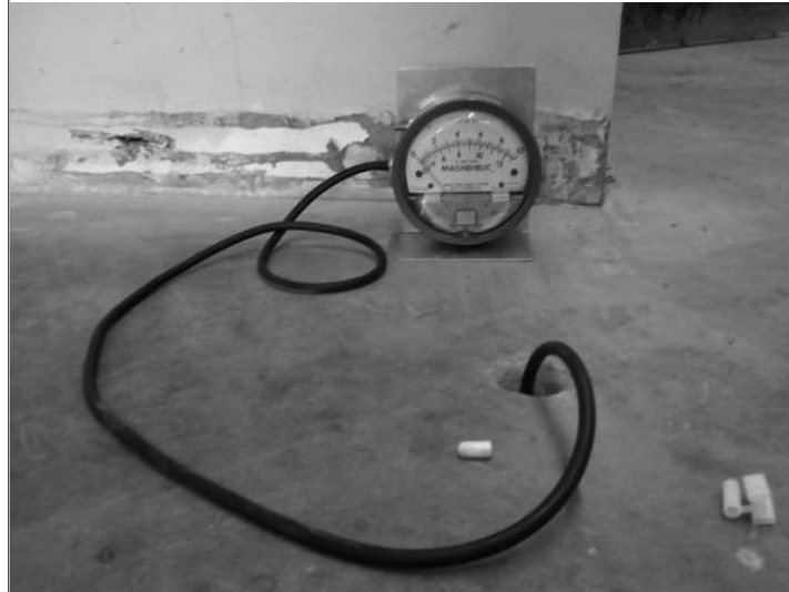
Title: Vapor Probe showing induced vacuum (0.2 inch water)
