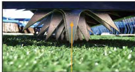
Height adjustable rotating tines between brushes to perforate and loosen infill
