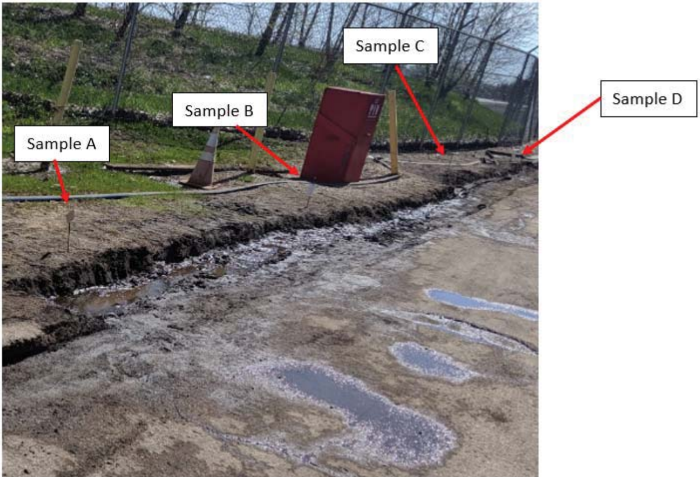
Pic 4 - Four soil samples were collected after initial soil was removed from the ground adjacent to asphalt. These sample results are detailed in the report. Similar locations where the TCLP sample was collected.
