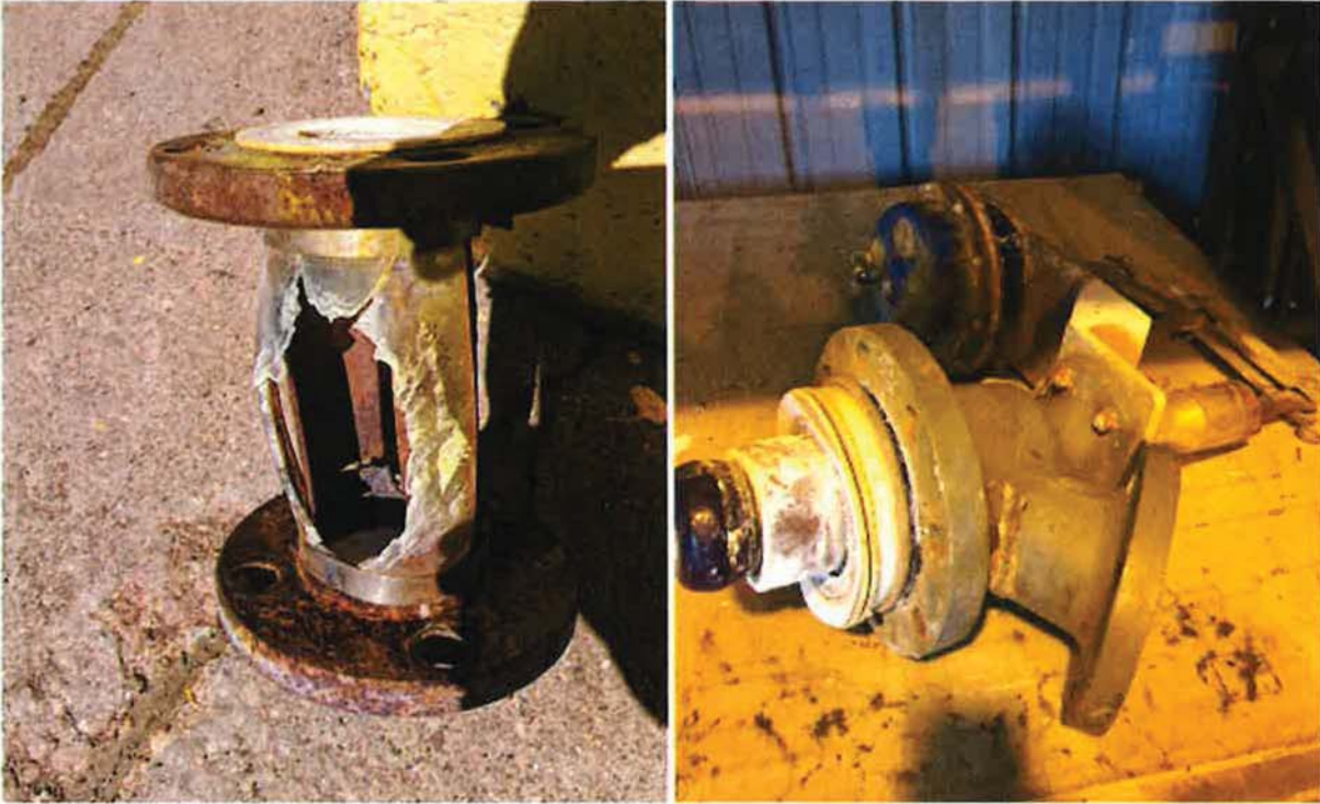
Pic 7 - Sight glass and Plug Valve
