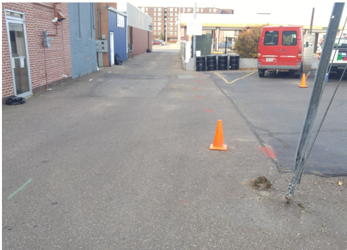
8. Photograph shows the alleyway from east to west. The near highway cone is over SP-16, while the farther cone is near SP-5/MW-1. The drums are associated with the installation and sampling of the wells.
