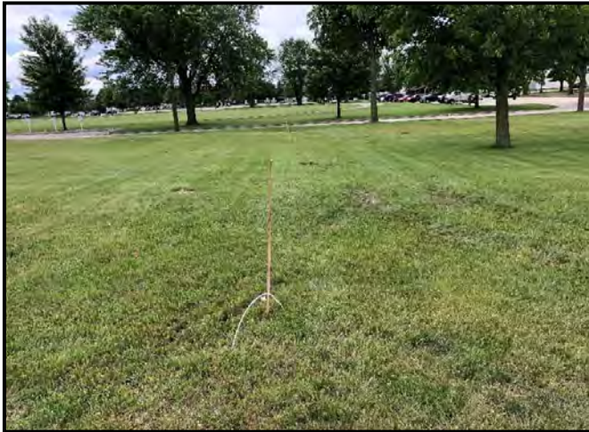
Temp wells installed in soil boring SB-2 and SB-3 after attempted sample collection.
