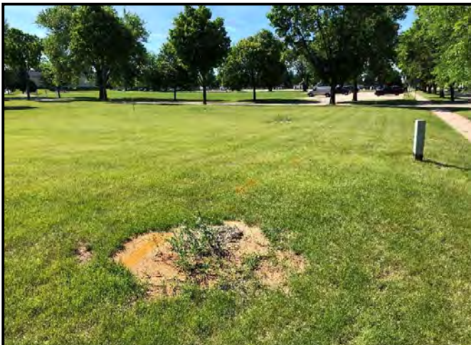
Marked utilities and abandoned previous soil boring locations.
