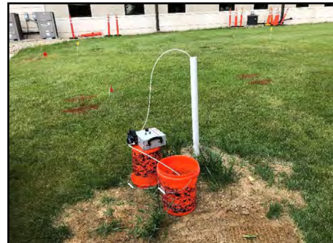
Groundwater sample collection from existing monitoring well.
