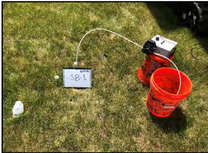
Groundwater sample collection SB-1.
