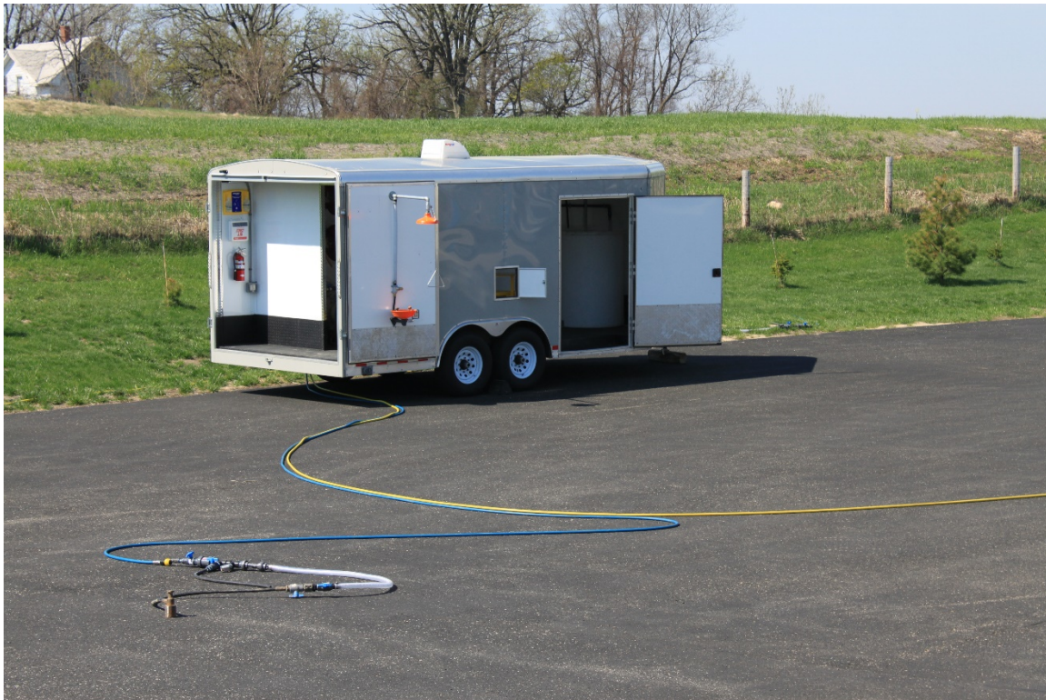
Figure 5 ORIN injection trailer.
