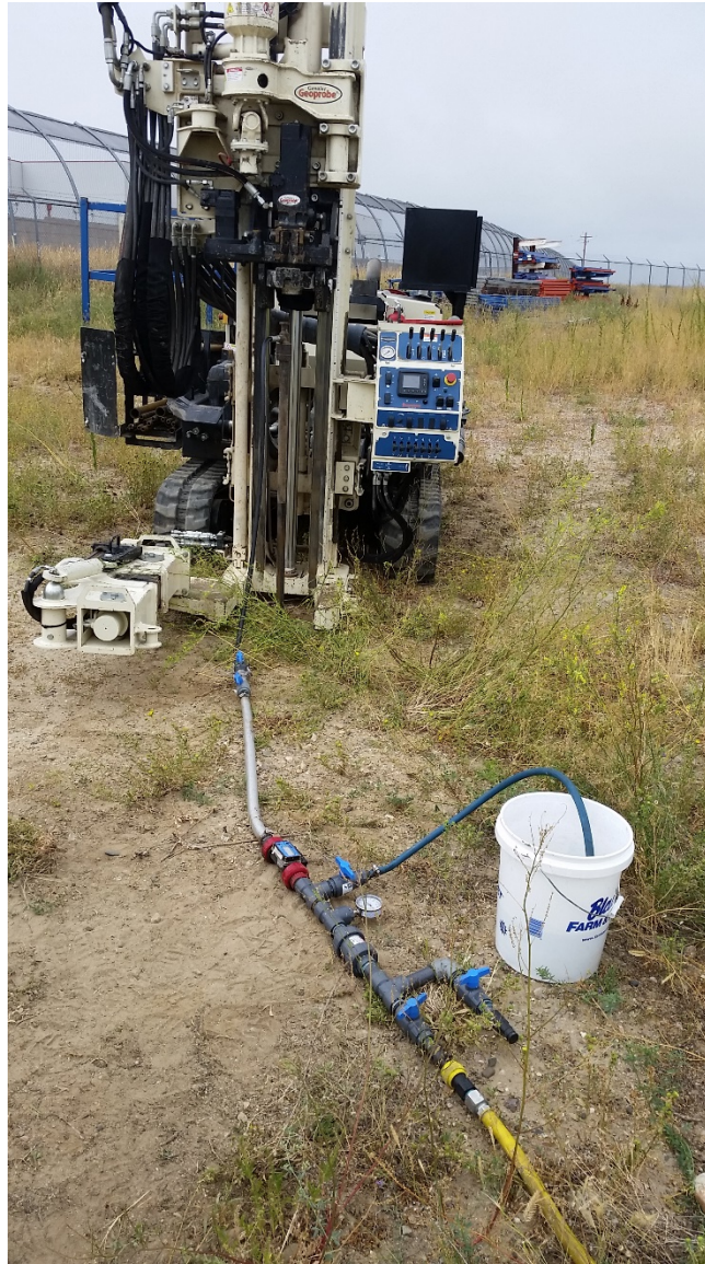
Figure 6 DPT Direct Push Technology in-situ injection.
