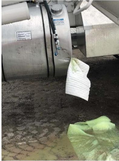
View of leaking saddle tank.
