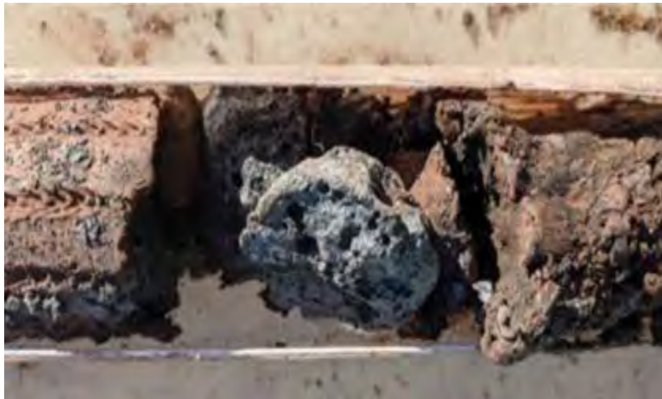
Photo 4: Slag like material in the 0.6-2 foot interval of SB-10.
