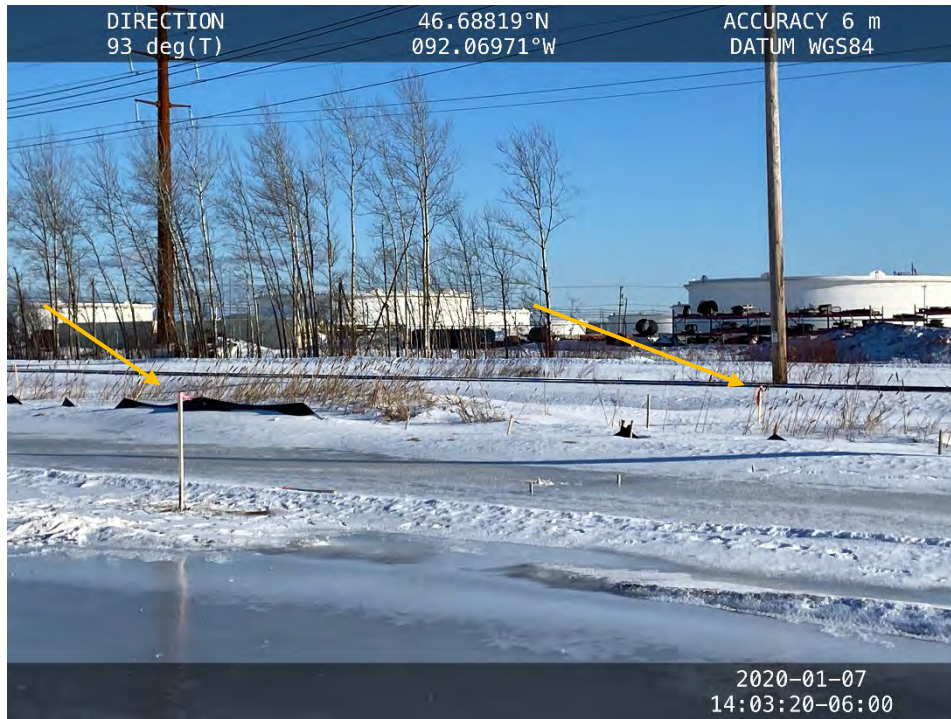
Photo 3: SB-18 offset 16 feet from original location. The original boring location is on the right side of the photo and the offset location is on the left.
