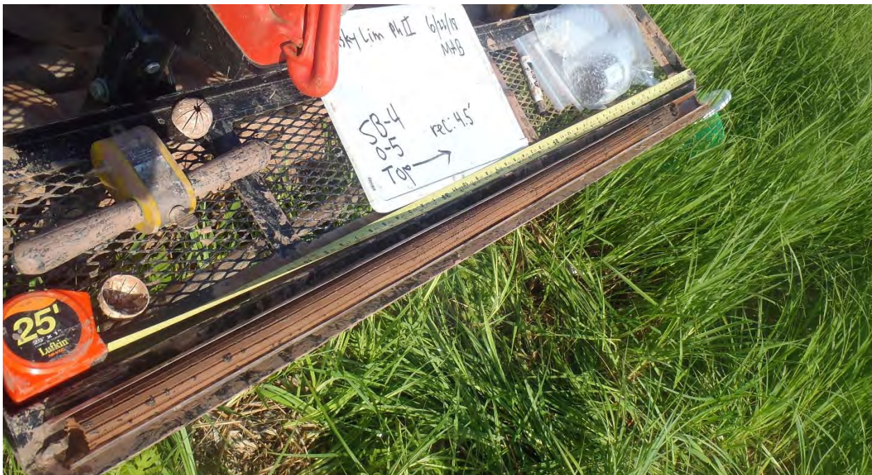
Photo 2: Typical soil boring recovery. Pictured is recovery from SB-4, 0-5 feet bgs. Thin layer of organic topsoil visible on right (top) end of sample sleeve. Soil below is stiff glaciolacustrine lean clay.
