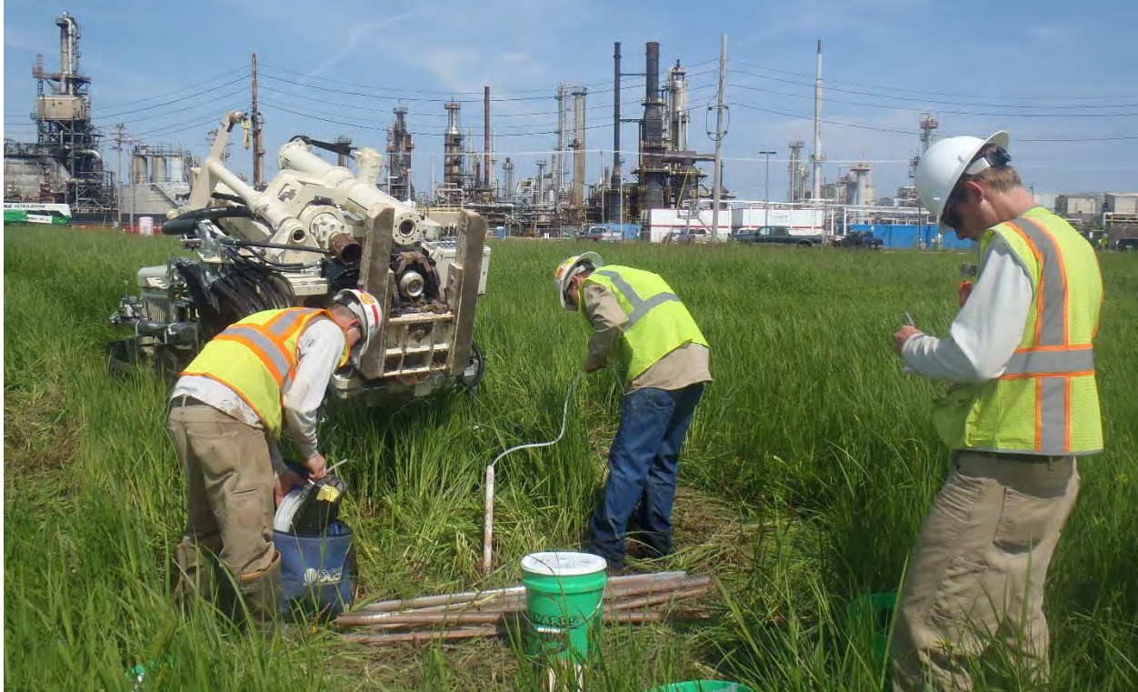
Photo 4: Attempting to sample the temporary monitoring well at SB-1.
