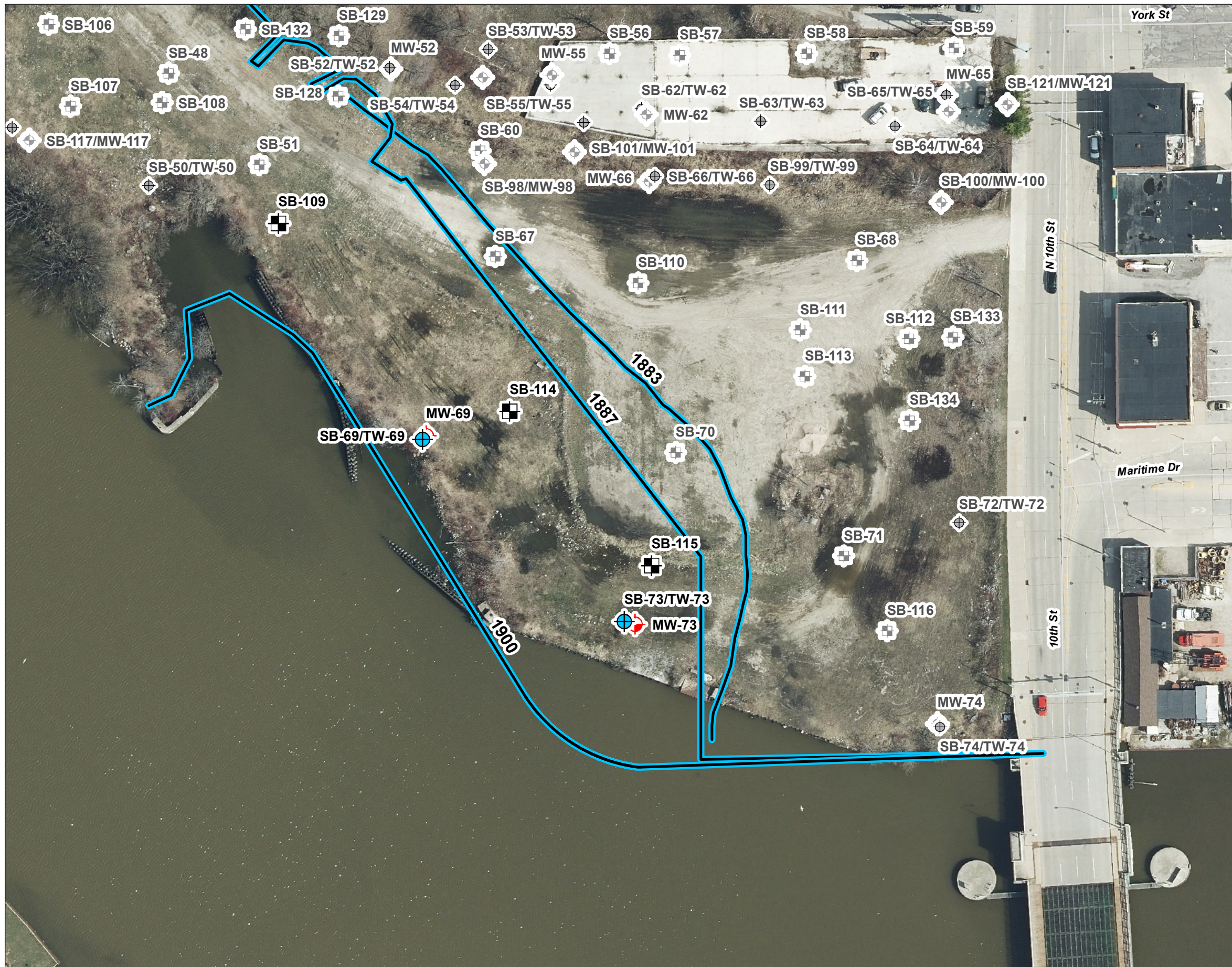
Figure No. 1 Title Sample Locations and the Historic Bank of the Manitowoc River
