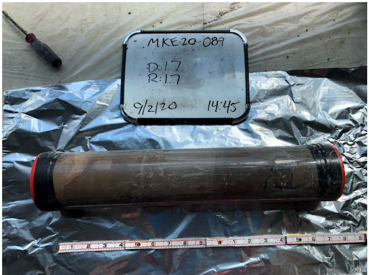
Photograph 1 MKE-20-089 (0.0–1.7 feet, intact core)
