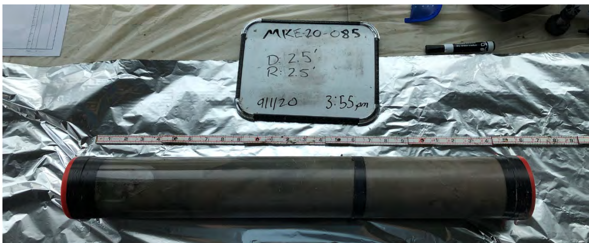
Photograph 1 MKE-20-085 (0.0–2.5 feet, intact core)
