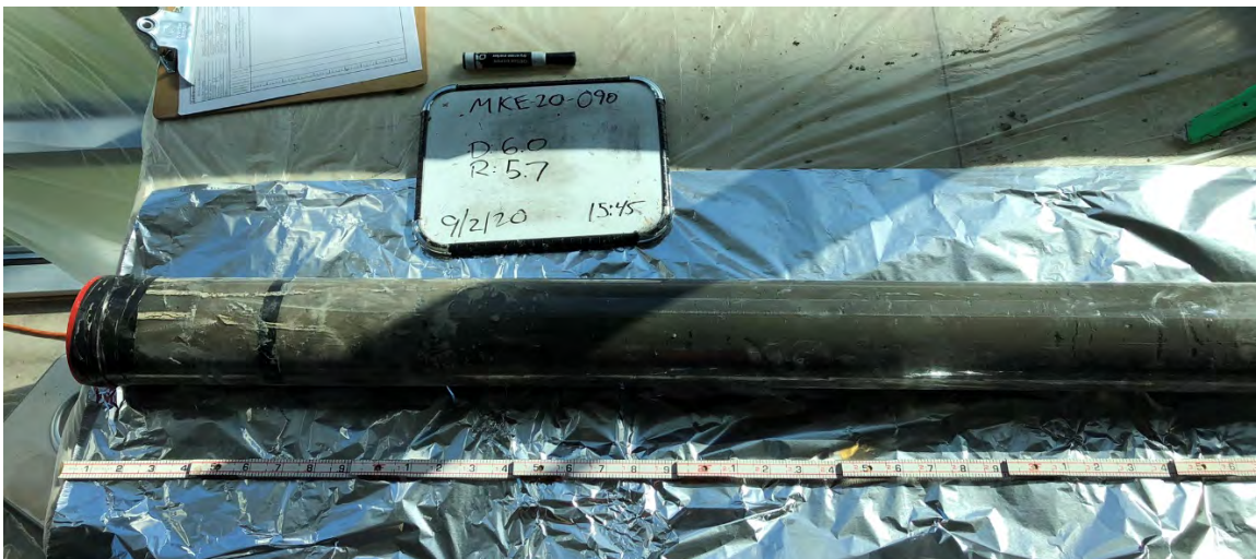
Photograph 2 MKE-20-090 (0.0–3.5 feet, intact core)
