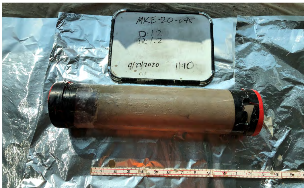
Photograph 1 MKE-20-095 (0.0–1.2 feet, intact core)
