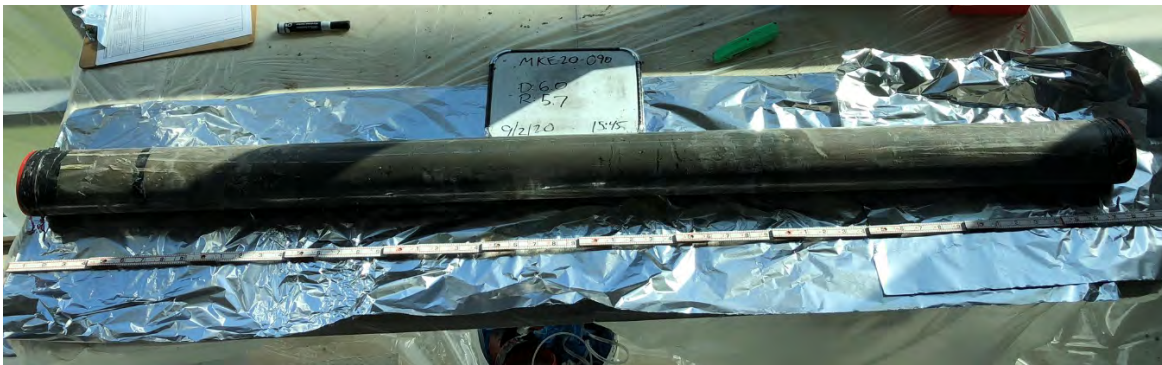
Photograph 1 MKE-20-090 (0.0–5.7 feet, intact core)
