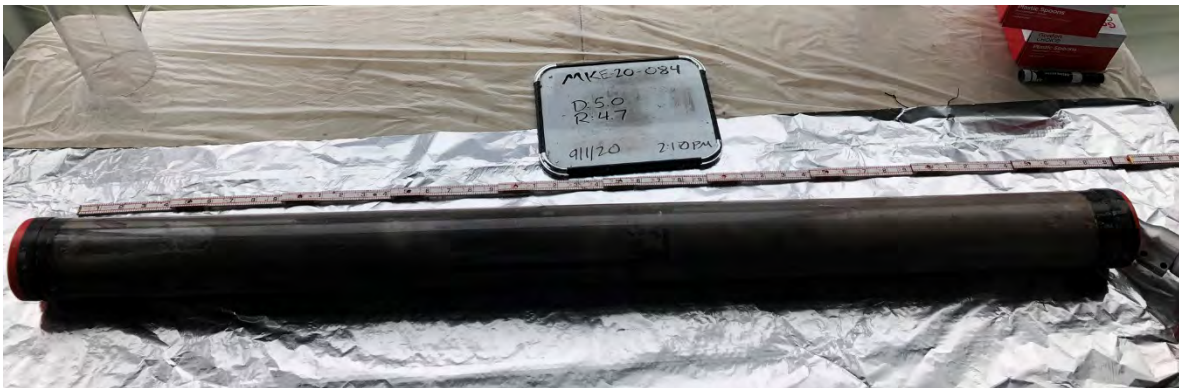
Photograph 1 MKE-20-084 (0.0–4.7 feet, intact core)
