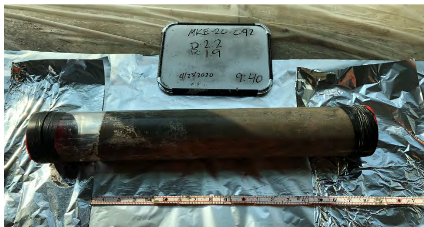
Photograph 1 MKE-20-092 (0.0–1.9 feet, intact core)
