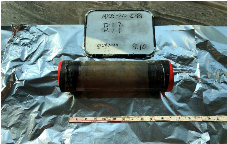
Photograph 1 MKE-20-081 (0.0–1.1 feet, intact core)
