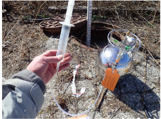
Figure 4 Purge teflon tubing with new syringe.
