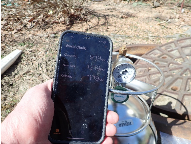
Figure 7 Starting vacuum reading on canister.
