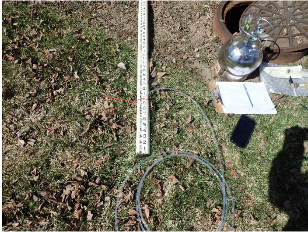
Figure 1 Teflon tubing held at set depth with wire ties.
