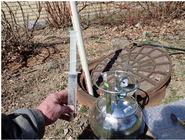
Figure 8 Purge teflon tubing with new syringe.
