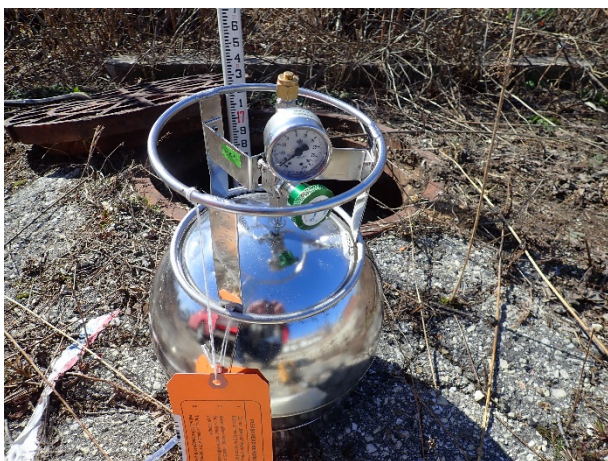
Figure 3 Starting vacuum reading on canister.
