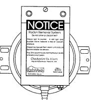
Cut a suitable length of vinyl tubing and attach it to the pressure switch connector on the CHECKPOINT IIa.
