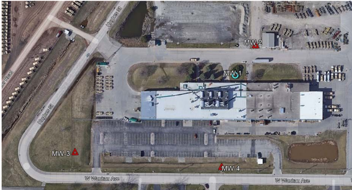
Figure 3. Proposed Soil Monitoring Well Locations. Existing Well (blue circle) and Proposed Wells (red triangle)
